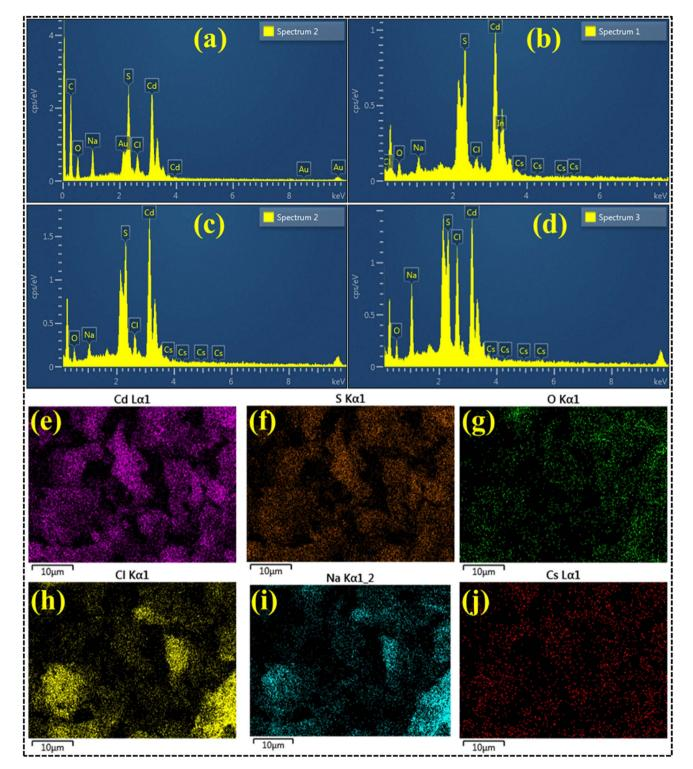
Fig. 5 EDS analysis of (a) CdS, (b) 1% CS doped CdS, (c) 3% CS doped CdS and (d) 5% CS doped CdS; (e-j) elemental mapping of 5% CS doped CdS QDs.
