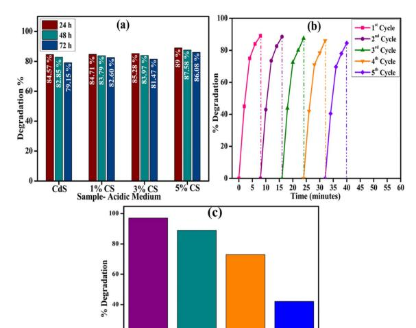
Fig. 10 (a) Stability and (b) reusability of the synthesized nanocatalyst for degradation of RhB dye in an acidic medium; (c) trapping experiment of active species during degradation of RhB.
