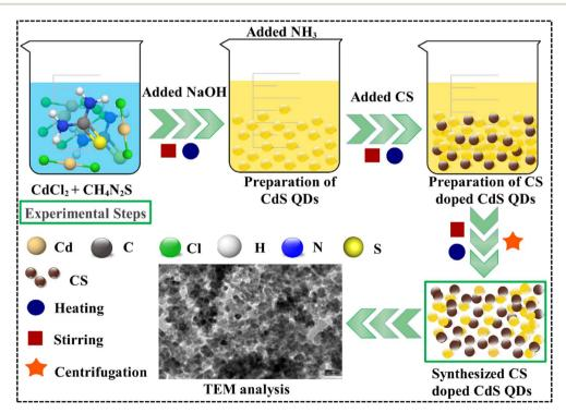
Fig. 1 Preparation of CS doped CdS QDs.
