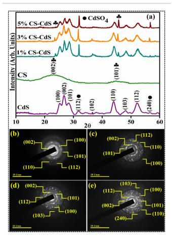
Fig. 3 (a) XRD and (b–e) SAED patterns of CdS, 1% CS doped CdS, 3% CS doped CdS, and 5% CS doped CdS QDs, respectively.
