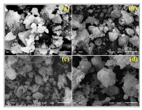
FESEM images of (a) CdS, (b) 1% CS doped CdS, (c) 3% CS doped CdS and (d) 5% CS doped CdS QDs
