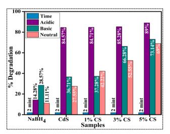
Catalytic reduction of RhB dye using the prepared nanocatalyst.
