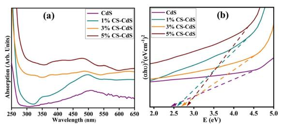
(a) Absorption spectra and (b)  $E_q$  by using the Tauc plot of pristine and CS doped CdS QDs.
