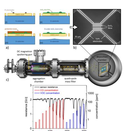
Fig. 1 (a) Fabrication steps for the realisation of CMOS-integrated SnO<sub>2</sub> thin films sensors. (b) Scanning electron microscopy image of typical device. The sensor structure is integrated on a suspended microhotplate mechanically connected via four arms. (c) Schematic of sensor functionalisation via magnetron-sputtering inert-gas condensation. (d) Chemoresistive signal of a pristine SnO<sub>2</sub>-based gas sensor at 50% relative humidity and an operation temperature of 200 °C.
