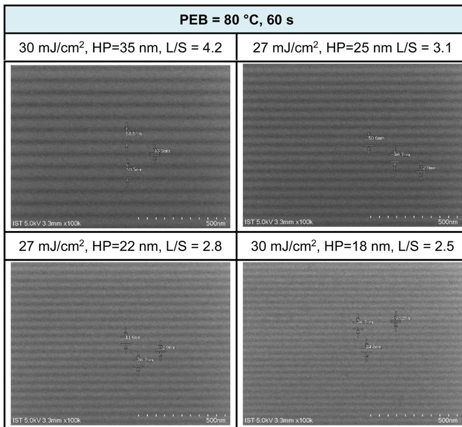
Fig. 8 SEM images of EUV lithographic patterns: THK = 24.5 nm, PAB (80 °C, 60 s, THK = 24.5 nm); developer: hexane/heptanone 1 : 1, 60 s.
