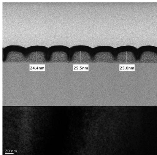
Fig. 10 Cross-section TEM image of an HP = 25 nm pattern ( $J = 109$  mJ cm<sup>-2</sup>).
