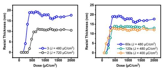
Fig. 4 E-beam contrast curves: left figure: 2.5 wt%, initial height 30.2 and 32 nm for clusters 3 and 2 respectively. Right figure: 2.5 wt% initial thickness 30.2 nm, PAB 80 °C, 60–180 s.
