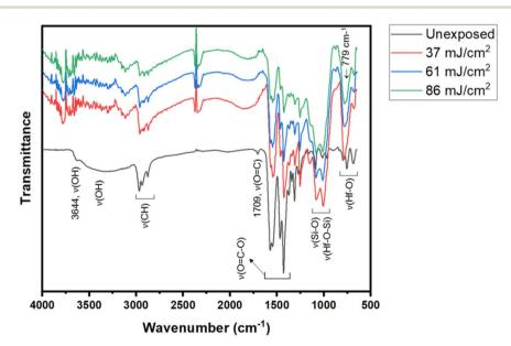
Fig. 13 FTIR spectra at different EUV doses; the intensities at J = 37-86 mJ cm<sup>-2</sup> were enlarged by 6 fold to show clarity.
