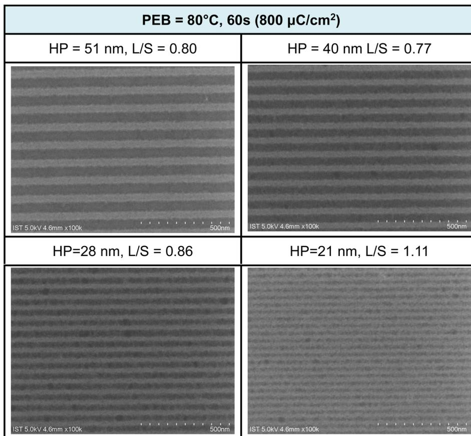
Fig. 6 SEM images of e-beam lithographic patterns for cluster 3 at different doses and half-pitches; the design is L/S = 1 : 1. PEB (80 °C, 60 s), developer: hexane/heptanone 1 : 1, 60 s. Initial film thickness 24.5 nm.
