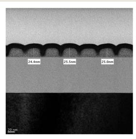
Fig. 10 Cross-section TEM image of an HP = 25 nm pattern (J = 109 $mJ cm^{-2}$ ).
