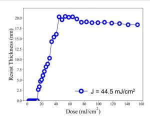
Fig. 7 EUV contrast curve; no PEB, initial thickness 24.5 nm.
