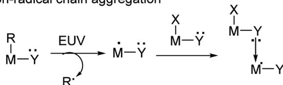
Scheme 1 Types of molecular aggregations for negative-tone photoresists.
