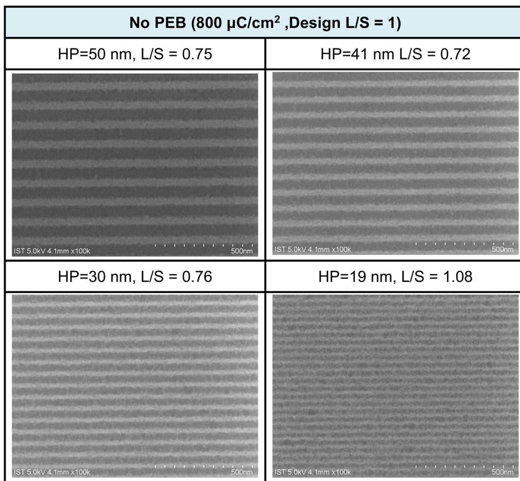
Fig. 5 SEM images of e-beam lithographic patterns for cluster 3 at different doses and half-pitches; the design is  $L/S = 1 : 1$ , developer: hexane/2-heptanone 1 : 1, 60 s. Initial film thickness 24.5 nm.
