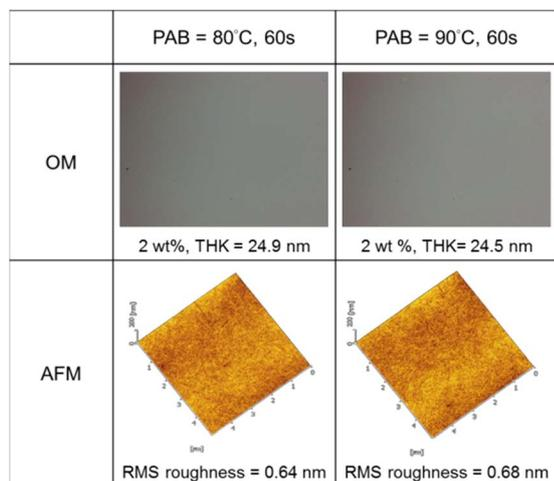
Fig. 3 Surface films of cluster 3 after solution spin-casting.
