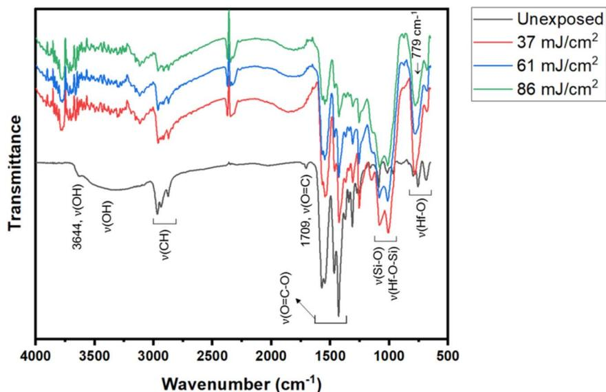
Fig. 13 FTIR spectra at different EUV doses; the intensities at  $J = 37\text{--}86$  mJ cm<sup>-2</sup> were enlarged by 6 fold to show clarity.
