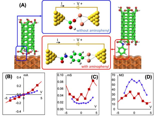
Fig. 5 (A) With and without aminophenyl models attached to nanogold electrodes for I-V curve calculations. The nanogold electrodes constitute the electron source and drain for the calculations. Nitrogen (blue), carbon (green), hydrogen (white), copper (orange), and gold (yellow). (B) I-V curves, (C) conductance, and (D) resistance of the with aminophenyl model (red curves) and without aminophenyl model (blue curves).
