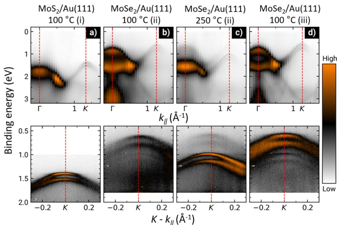
**Fig. 4** Angle-resolved UP spectra of (a) MoS<sub>2</sub> (i) annealed at 100 °C, MoSe<sub>2</sub> (ii) annealed at (b) 100 °C and (c) 250 °C as well as (d) MoSe<sub>2</sub> (iii) on Au(111) annealed at 100 °C. In the top parts, the band structures along  $\Gamma$ - $K$  direction are shown. Below, detailed parts of the band structure acquired with the 2D detector around the  $K$  points are presented.
