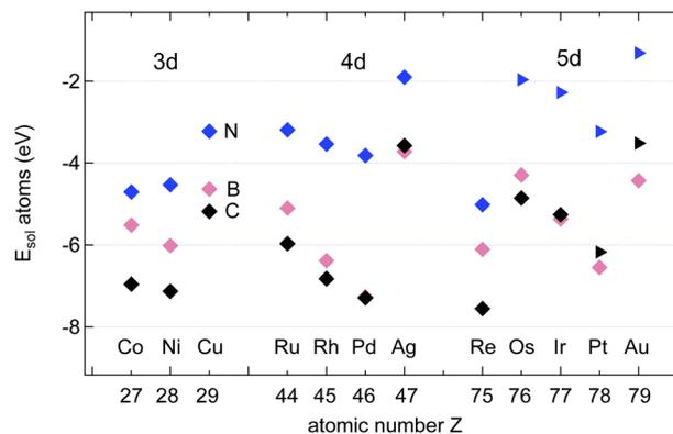
Fig. 3 Calculated solvation energies  $E_{\text{sol}}^{\text{A}}$ . A = B (pink), N (blue) and C (black) into the bulk of 12 different transition metals as a function of their atomic numbers. The symbols depict the octahedral  $\diamond$  or tetrahedral  $\triangleright$  sites. Data adapted from ref. 13.
