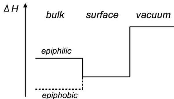
Fig. 2 Scheme of the enthalpies  $\Delta H$  involved in gas–solid reactions. In the epiphilic case the reactant has the lowest energy at the surface, while for the epiphobic case, the dissolution into the bulk is energetically favourable.
