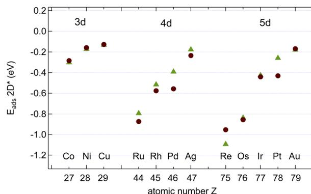
**Fig. 7** Calculated energies  $E_{\text{ads}}^{\text{AB}}$  of graphene (brown circles) and h-BN (green triangles) on the studied surfaces. The energy reference is graphene or h-BN strained to the lattice constant of the corresponding transition metal. Except for Re (B, N = C, C = hcp, top) and Au (B, N = C, C = top, fcc) all registries are (B, N = C, C = fcc, top).
