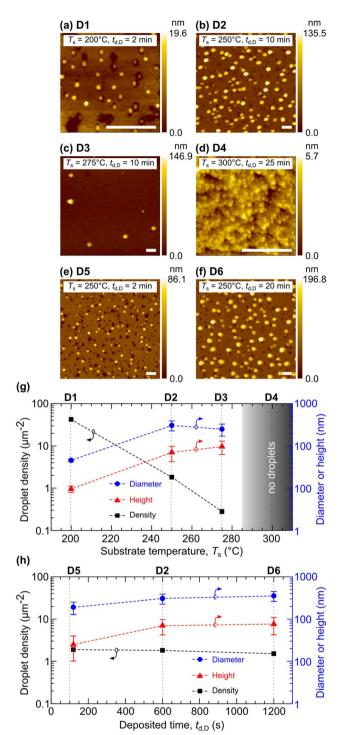
Fig. 1 (a)-(f) AFM images of Bi droplets synthesized at various substrate temperatures ( $T_{\rm s}$ ) and deposition times ( $t_{\rm d,D}$ ). Scale bars in (a)–(f) correspond to 0.5 μm. (g) Variations of droplet heights, diameters, and droplet densities as a function of  $T_s$  for samples D1, D2, and D3. (h) Variations of droplet heights, diameters, and droplet densities as a function of  $t_{d,D}$  for samples D2, D5, and D6.
