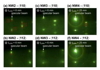
Fig. 5 (a)-(f) RHEED diffraction patterns recorded along the (110) and (112) azimuths during the growth of NW2, NW3, and NW4. The images were snapped at different GaAsBi nanowire deposition times ( $t_{d,NW}$ ) as provided in each panel.
