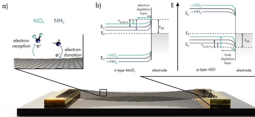
Fig. 1 Gas sensing mechanisms on a semiconducting material, such as a graphene derivative; (a) electron exchange between gas molecules and receptor; (b) shift of the band structure at the semiconductor-electrode contact.
