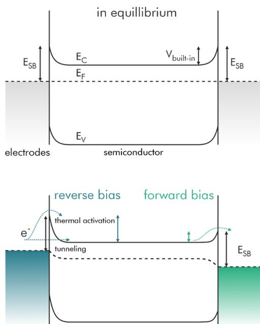
Fig. 2 Typical band diagram of a double-Schottky barrier device in unbiased and biased condition. A potential is applied to the left contact. Electrons flow from left to right; redrawn and adapted, with permission from ref. 39.
