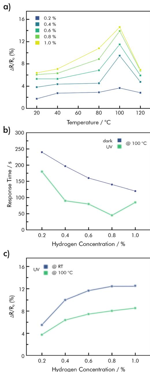
Fig. 11 Hybrid Pd/rGO sensing performance (a) temperature-dependent responses towards H<sub>2</sub> at different concentrations; (b) effect of UV-illumination on response times as a function of H<sub>2</sub>-concentration at 100 °C; (c) signal responses under UV-illumination at RT and 100 °C as a function of H<sub>2</sub>-concentration; redrawn with data from ref. 82.
