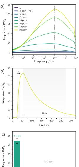
Fig. 12 Hybrid NFI-rGO sensing performance (a) relative response variation as a function of frequency for NH<sub>3</sub> concentrations from 0-60 ppm; (b) dynamic response-recovery curve for exposure to 60 ppm of NH<sub>3</sub>; (c) cross-sensitivity between NH<sub>3</sub> (15 ppm), acetone, ethanol, methanol, monomethylamine (MMA), trimethylamine (TMA) and triethylamine (TEA) (150 ppm); redrawn and adapted, with permission from ref. 146
