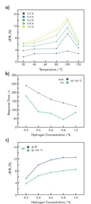
Fig. 11 Hybrid Pd/rGO sensing performance (a) temperaturedependent responses towards H<sub>2</sub> at different concentrations; (b) effect of UV-illumination on response times as a function of H<sub>2</sub>concentration at 100 °C; (c) signal responses under UV-illumination at RT and 100 °C as a function of H<sub>2</sub>-concentration; redrawn with data from ref. 82.
