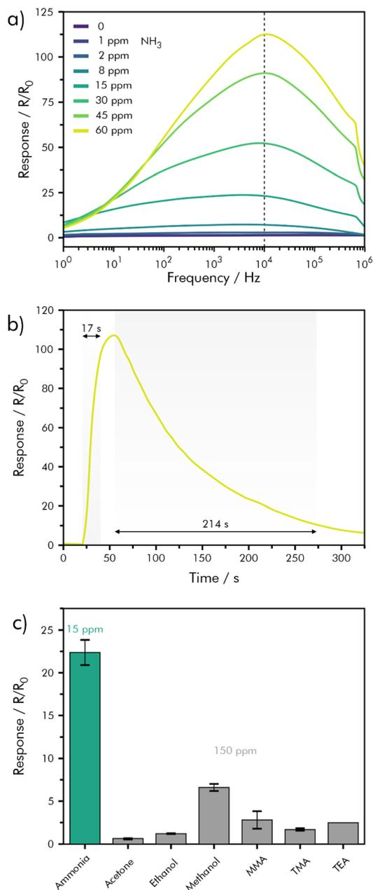
Fig. 12 Hybrid NFI-rGO sensing performance (a) relative response variation as a function of frequency for  $\text{NH}_3$  concentrations from 0–60 ppm; (b) dynamic response–recovery curve for exposure to 60 ppm of  $\text{NH}_3$ ; (c) cross-sensitivity between  $\text{NH}_3$  (15 ppm), acetone, ethanol, methanol, monomethylamine (MMA), trimethylamine (TMA) and triethylamine (TEA) (150 ppm); redrawn and adapted, with permission from ref. 146.
