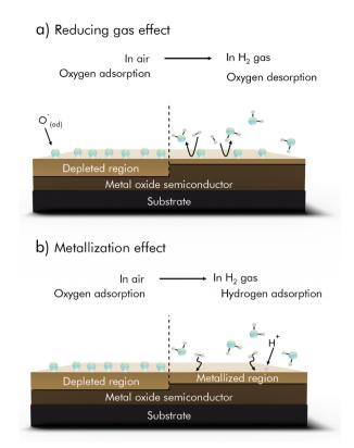
Fig. 4 H<sub>2</sub> sensing mechanisms of MOx based H<sub>2</sub> sensors. (a) Reducing gas effect. (b) Metallization effect; reprinted (adapted) with permission from ref. 43. Copyright 2020 American Chemical Society.
