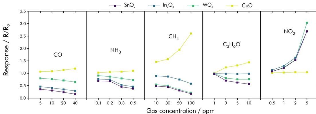
Fig. 15 Signal responses and sample variations of  $\text{SnO}_2$ ,  $\text{In}_2\text{O}_3$ ,  $\text{WO}_3$  and  $\text{CuO}$  towards  $\text{CO}$ ,  $\text{NH}_3$ ,  $\text{CH}_4$ , acetone and  $\text{NO}_2$ ; reprinted (adapted) with permission from ref. 162. Copyright 2022 American Chemical Society.
