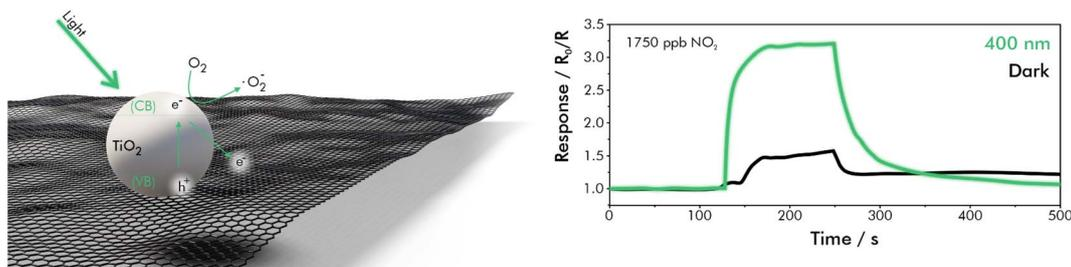
Fig. 10 Sensing mechanism and dynamic response–recovery curves of GTiO<sub>2</sub>S towards 1750 ppb of NO<sub>2</sub> in dark and illuminated operating mode; redrawn and adapted from ref. 138.
