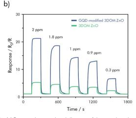
Fig. 14 (a) Proposed energy band diagram of the p-n-junction at the interface of 3DOM ZnO and GQD; (b) dynamic response curves for 3DOM ZnO and GQD-modified 3DOM ZnO in the concentration range 0.3–2 ppm acetone; redrawn and adapted, with permission from ref. 152.
