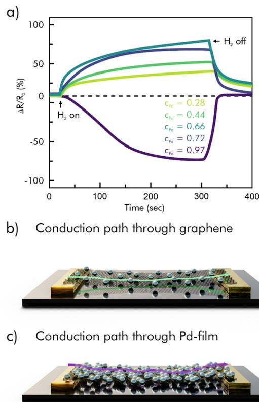
Fig. 7 a) Relative resistance response (shown in percent) of PMMA/Pd/graphene hybrid sensors with different values of  $c_{Pd}$  on single-layer graphene as a function of time, exposed to 2% H<sub>2</sub>; (b and c) schematic representation of the conduction path through graphene and Pd; reprinted (adapted) with permission from ref. 113. Copyright 2015 American Chemical Society.
