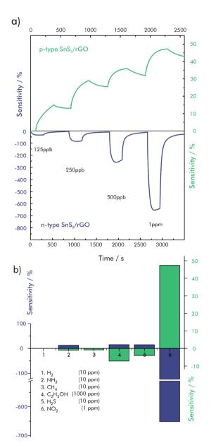
Fig. 8 Gas sensing performances of n-type  $SnS_2/rGO$  and p-type  $SnS_2/rGO$ ; (a) dynamic response–recovery curves towards  $NO_2$  at concentrations from 125 ppb to 1 ppm at RT, (b) cross sensitivity of  $NO_2$  (1 ppm) towards  $H_2$  (10 ppm),  $NH_3$  (10 ppm),  $CH_4$  (10 ppm),  $C_2H_5OH$  (1000 ppm) and  $H_2S$  (10 ppm); redrawn and adapted, with permission from ref. 103.
