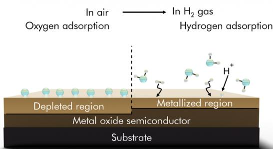
Fig. 4 H<sub>2</sub> sensing mechanisms of MO<sub>x</sub> based H<sub>2</sub> sensors. (a) Reducing gas effect. (b) Metallization effect; reprinted (adapted) with permission from ref. 43. Copyright 2020 American Chemical Society.
