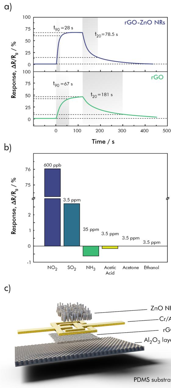
**Fig. 9** (a) Dynamic response recovery curves from rGO and the rGO-ZnO NR towards  $\text{NO}_2$  at a concentration of 400 ppb, (b) selectivity test using  $\text{NO}_2$  (600 ppb),  $\text{SO}_2$  (3.5 ppm),  $\text{NH}_3$  (35 ppm), acetic acid (3.5 ppm), acetone (3.5 ppm), and ethanol (3.5 ppm); (c) sensor geometry of the stacked rGO-ZnO NR hybrid sensor; redrawn and adapted, with permission from ref. 130.
