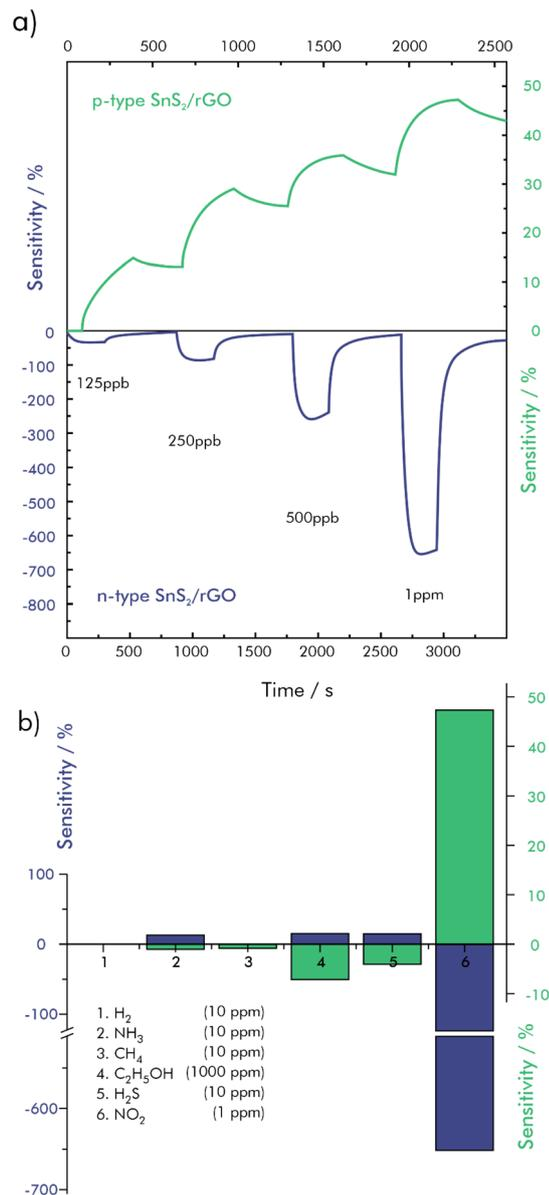
**Fig. 8** Gas sensing performances of n-type  $\text{SnS}_2/\text{rGO}$  and p-type  $\text{SnS}_2/\text{rGO}$ ; (a) dynamic response–recovery curves towards  $\text{NO}_2$  at concentrations from 125 ppb to 1 ppm at RT, (b) cross sensitivity of  $\text{NO}_2$  (1 ppm) towards  $\text{H}_2$  (10 ppm),  $\text{NH}_3$  (10 ppm),  $\text{CH}_4$  (10 ppm),  $\text{C}_2\text{H}_5\text{OH}$  (1000 ppm) and  $\text{H}_2\text{S}$  (10 ppm); redrawn and adapted, with permission from ref. 103.
