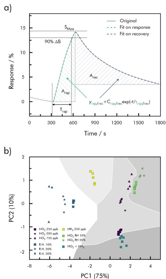
Fig. 16 (a) Feature extraction from the gas response curve (red and blue lines are the exponential fitted curves for the response and recovery regime); (b) decision map for  $\text{NO}_2$ , humid air,  $\text{NH}_3$ ,  $\text{NO}_2$  under humid air, and a mixture of  $\text{NO}_2$  and  $\text{NH}_3$  classified by applying *k*-nearest neighbor (*k*NN) to the PCA model with *k* = 5; redrawn and adapted from ref. 164.
