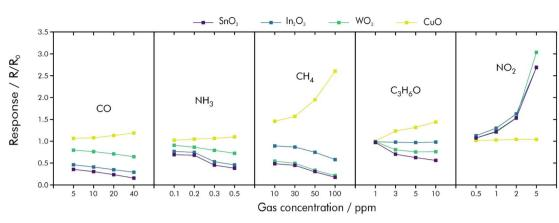
Fig. 15 Signal responses and sample variations of  $SnO_2$ ,  $In_2O_3$ ,  $WO_3$  and CuO towards CO,  $NH_3$ ,  $CH_4$ , acetone and  $NO_2$ ; reprinted (adapted) with permission from ref. 162. Copyright 2022 American Chemical Society.
