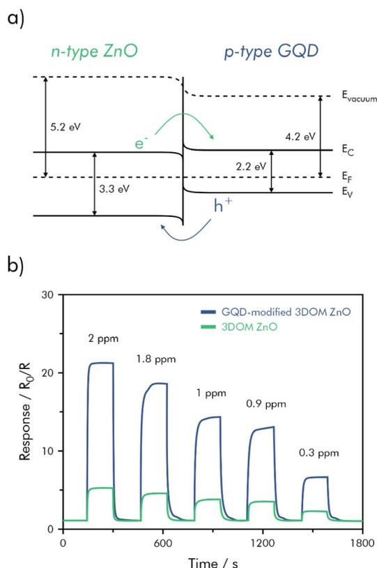
**Fig. 14** (a) Proposed energy band diagram of the p–n-junction at the interface of 3DOM ZnO and GQD; (b) dynamic response curves for 3DOM ZnO and GQD-modified 3DOM ZnO in the concentration range 0.3–2 ppm acetone; redrawn and adapted, with permission from ref. 152.
