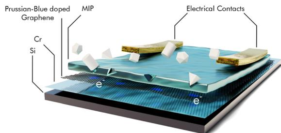
**Fig. 13** 4-layer structure of the VOC sensor with electrical contacts to be connected to a printed circuit board, target molecules are trapped inside the cavities of the MIP and the extra electron is transferred to the graphene layer causing a resistance change; redrawn and adapted, with permission from ref. 158.
