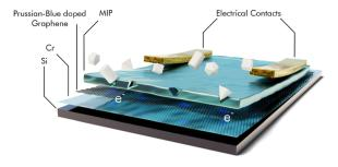
Fig. 13 4-layer structure of the VOC sensor with electrical contacts to be connected to a printed circuit board, target molecules are trapped inside the cavities of the MIP and the extra electron is transferred to the graphene layer causing a resistance change; redrawn and adapted, with permission from ref. 158.
