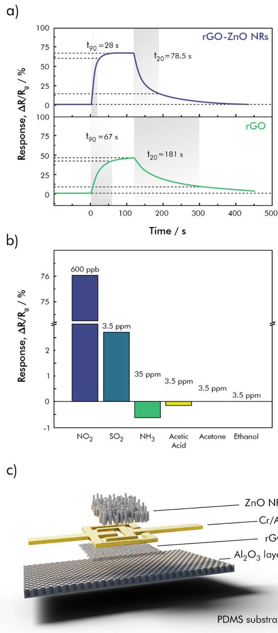
**Fig. 9** (a) Dynamic response recovery curves from rGO and the rGO-ZnO NR towards NO<sub>2</sub> at a concentration of 400 ppb, (b) selectivity test using NO<sub>2</sub> (600 ppb), SO<sub>2</sub> (3.5 ppm), NH<sub>3</sub> (35 ppm), acetic acid (3.5 ppm), acetone (3.5 ppm), and ethanol (3.5 ppm); (c) sensor geometry of the stacked rGO-ZnO NR hybrid sensor; redrawn and adapted, with permission from ref. 130.
