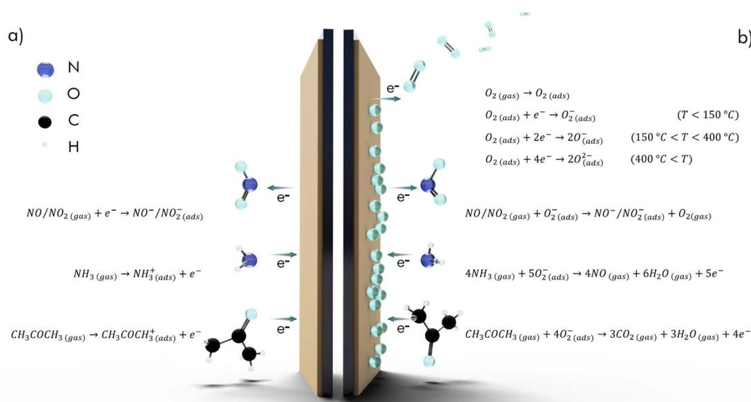
Fig. 3 Reaction equations for  $NO_2$ ,  $NH_3$  and acetone on a semiconducting sensor substrate with inert gas (a) and air (b) as support gas. Temperature dependent oxygen adsorption applies to MOx sensors.
