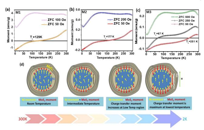
Fig. 3 Spontaneous magnetization as a function of temperature with various ZFC magnetic fields for (a) M1, (b) M2 and (c) M3 composites.  $T_c$  represents the compensation temperature that varies with the samples. (d) Schematic model for change of spin alignment at the interface in the hybrid nanostructure with temperature changes. The magnitudes of the Ni moment and  $MoS_2$  moment change with temperature. Red and yellow represent the spin magnetic moments from  $MoS_2$  and Ni, respectively.
