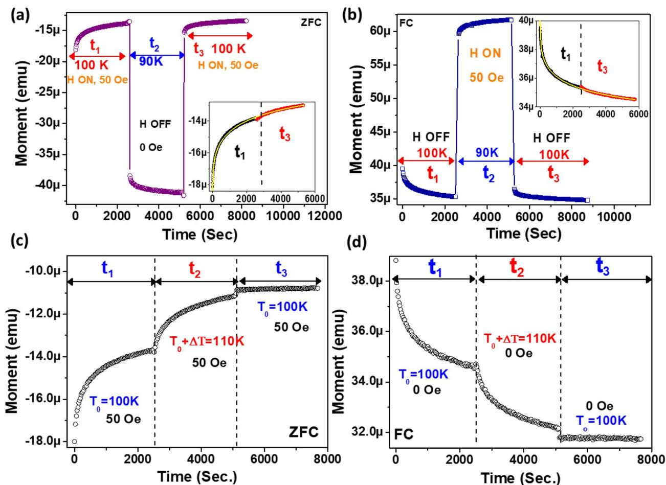
Fig. 7 (a and b) Forced relaxations with simultaneous temperature and field changes for (a) the ZFC method and (b) the FC method. The inset shows that  $t_3$  is a continuation of  $t_1$  fitted with eqn (1), even after a large jump. (c and d) Magnetic relaxation with positive thermal cycling for (c) the ZFC method and (d) the FC method. Reinitialization of the memory state occurs with  $\Delta T$  positive thermal cycling. Here,  $t_3$  is not a continuation of  $t_1$ .
