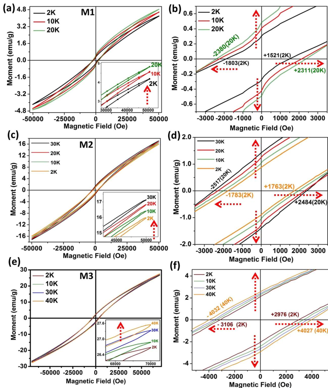
Fig. 4  $M-H$  hysteresis loops at different temperatures. (a) For M1; inset shows the increasing moment value with temperature. (b) Magnified view for M1 showing increasing coercivity and remanent magnetization with temperature, up to 20 K. (c)  $M-H$  loop for M2. (d) Increasing coercivity and remanent magnetization with temperature, up to 30 K. (e)  $M-H$  loop for M3. (f) Magnified view shows increasing coercivity and remanent magnetization with temperature, up to 40 K.
