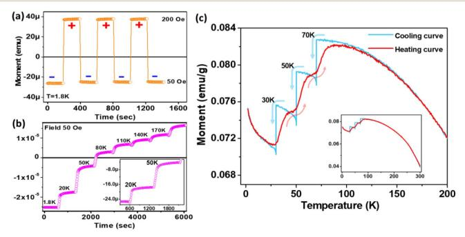
Fig. 5 (a) Switching polarity of magnetization response with applied field bias. (b) Transient response of magnetization with changing temperature at constant field. (c) Thermoremanent magnetization history, showing the memory effect, and retracing cooling and heating curves at the particular states. The inset shows the full-view curve in the temperature range of 1.8–300 K.
