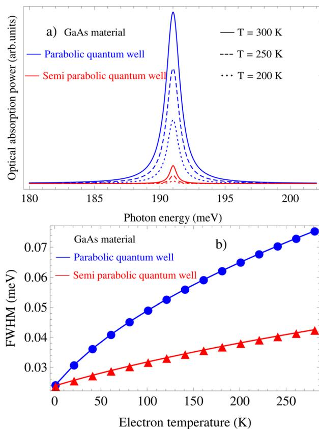
**Fig. 2** (a) Photon-energy dependence of the acoustic-phonon-assisted CR absorption power at the CR-peak with the inter-sub-band transition for different electron temperatures in the parabolic and semi-parabolic QWs for a typical GaAs material at a magnetic field of 10 T. (b) Dependence of the EAP interaction strength in the parabolic and semi-parabolic QWs for a typical GaAs material on the electron temperature at a magnetic field of 10 T.
