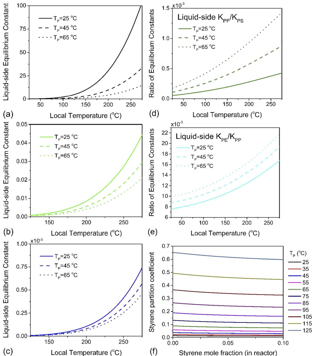
Fig. 5 The liquid-side equilibrium constant  $K_1$  as a function of depolymerization temperature for (a) PS, (b) PP and (c) PE at average particle temperatures of  $T_p = 298\text{ K}$ ,  $318\text{ K}$  and  $338\text{ K}$ , and at each of these temperatures, the ratio of  $K_1$ 's (d) for PP over PS and (e) for PE over PP. (f) Partition coefficient  $\pi_m$  of styrene defined in eqn (12) as a function of styrene mole fraction for various PS particle temperatures.
