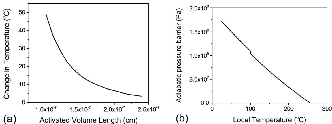
Fig. 4 PS depropagation proceeding along mostly thermal or mostly adiabatic compression mechanisms; (a) solution to eqn (10) – activated volume length  $\lambda$  versus change in temperature  $\Delta T$  within the volume  $\lambda^3$  assuming isothermal depropagation, (b) energy barrier for depropagation in the adiabatic compression mechanism expressed as a pressure (energy density) versus temperature.
