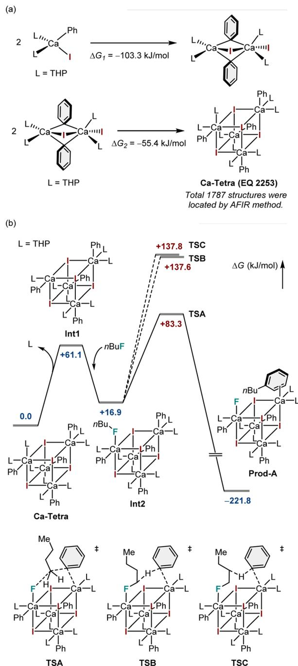
Fig. 1 Theoretical calculations to reveal the plausible structure of PhCaI(THP)<sub>2</sub> in solid state and the mechanism of the defluorinated C-C cross-coupling reaction (energies are given in kJ mol<sup>-1</sup>). (a) Stability of calcium species. (b) Energy profiles of possible reaction pathways.
