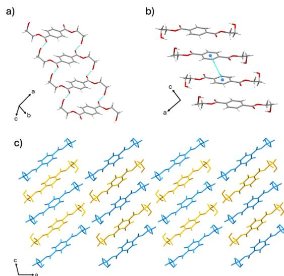
Fig. 1 Crystal structure of the  $\alpha$  form showing: (a) hydrogen bonding, (b) offset  $\pi$ – $\pi$  stacking, and (c) extended crystal structure packing (molecules colored blue and yellow for visual clarity).
