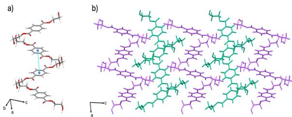
Fig. 2 Crystal structure of the  $\delta$  form showing: (a) hydrogen bonding and offset  $\pi$ - $\pi$  stacking, and (b) extended crystal structure packing (molecules colored magenta and teal for visual clarity).
