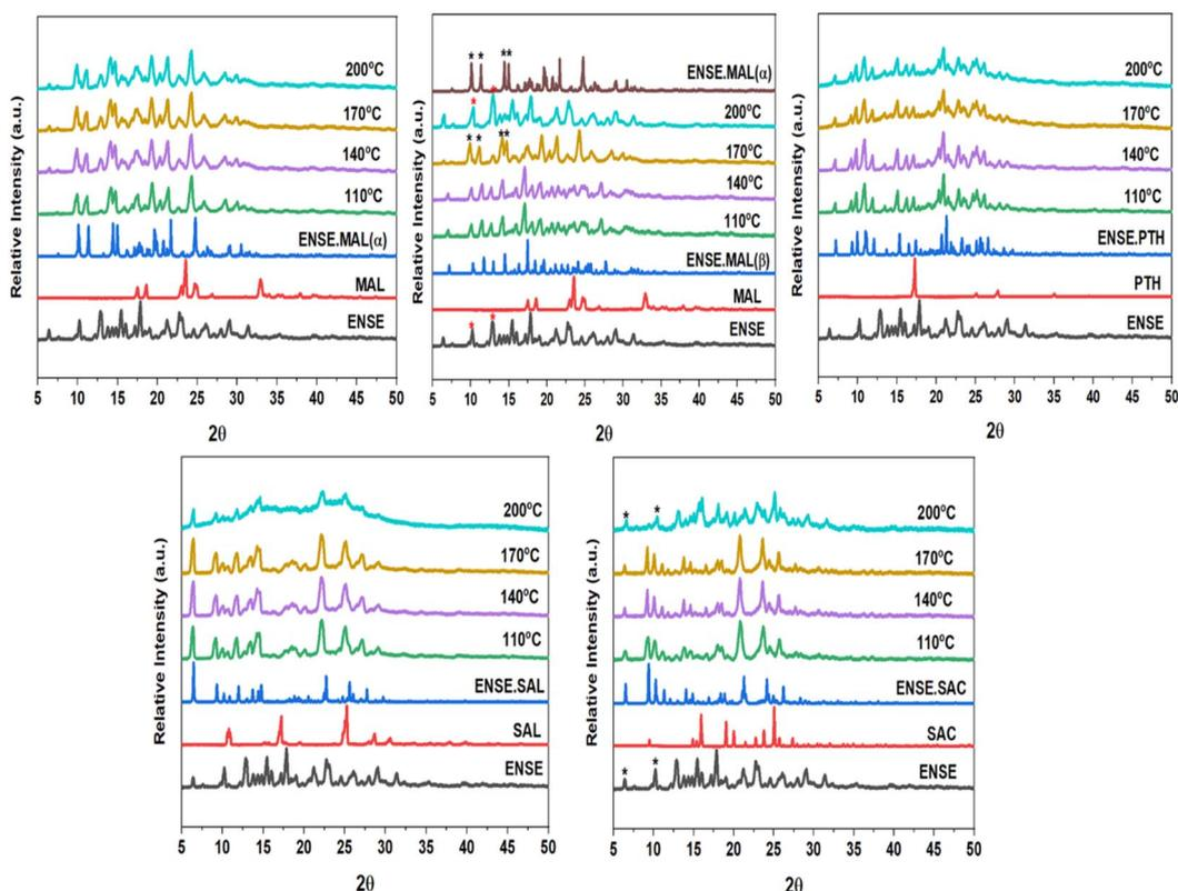
Fig. 8 VT-PXRD overlay of different adducts of ENSE.
