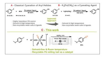
Scheme 1 Cyanation of aryl halides. (A) Early developed transition metal catalyzed cyanation of aryl halides. (B) First reported potassium ferrocyanide-based cyanation of aryl halide by Beller's group. (C) Proposed model scheme of direct mechanochemical cyanation reaction using potassium ferrocyanide.
