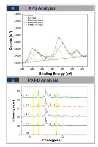
Fig. 3 (a) XPS analysis of the reaction mixture under the optimized reaction conditions (Fig. 1(E), entry 3). (b) Time dependent PXRD analysis of the optimized reaction conditions (Fig. 1(E), entry 3).
