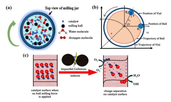
Fig. 9 (a) Top view representation of ball milling jar, (b) trajectory of balls in milling jar, and (c) schematic representation showing production of reactive species when STO gets trapped between two balls during collision.
