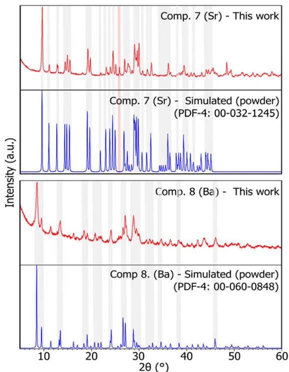
Fig. 8 X-ray diffraction patterns of compounds **7** and **8** (Sr, and Ba), respectively. Red: sample pattern obtained in this work. Blue: simulated pattern from powder data obtained from the PDF-4 database.<sup>24</sup> Some shaded areas are in place between corresponding experimental and simulated patterns for easier comparison. The red shaded area highlights a peak of  $\text{MoO}_3$ . The reader is referred to the digital version of this article for the colour version of the figure.
