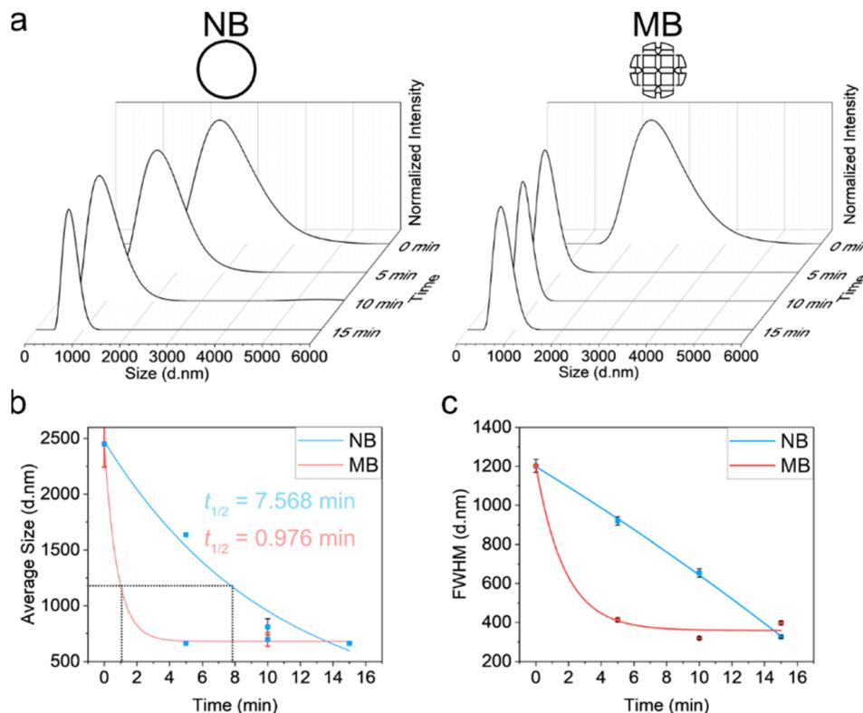
Fig. 5 (a) DLS of TiO<sub>2</sub> treated with PBM using NB or MB. (b) Average size of milled particles derived from DLS data. (c) FWHM analysis derived from average particle size distribution of milled nanoparticles.
