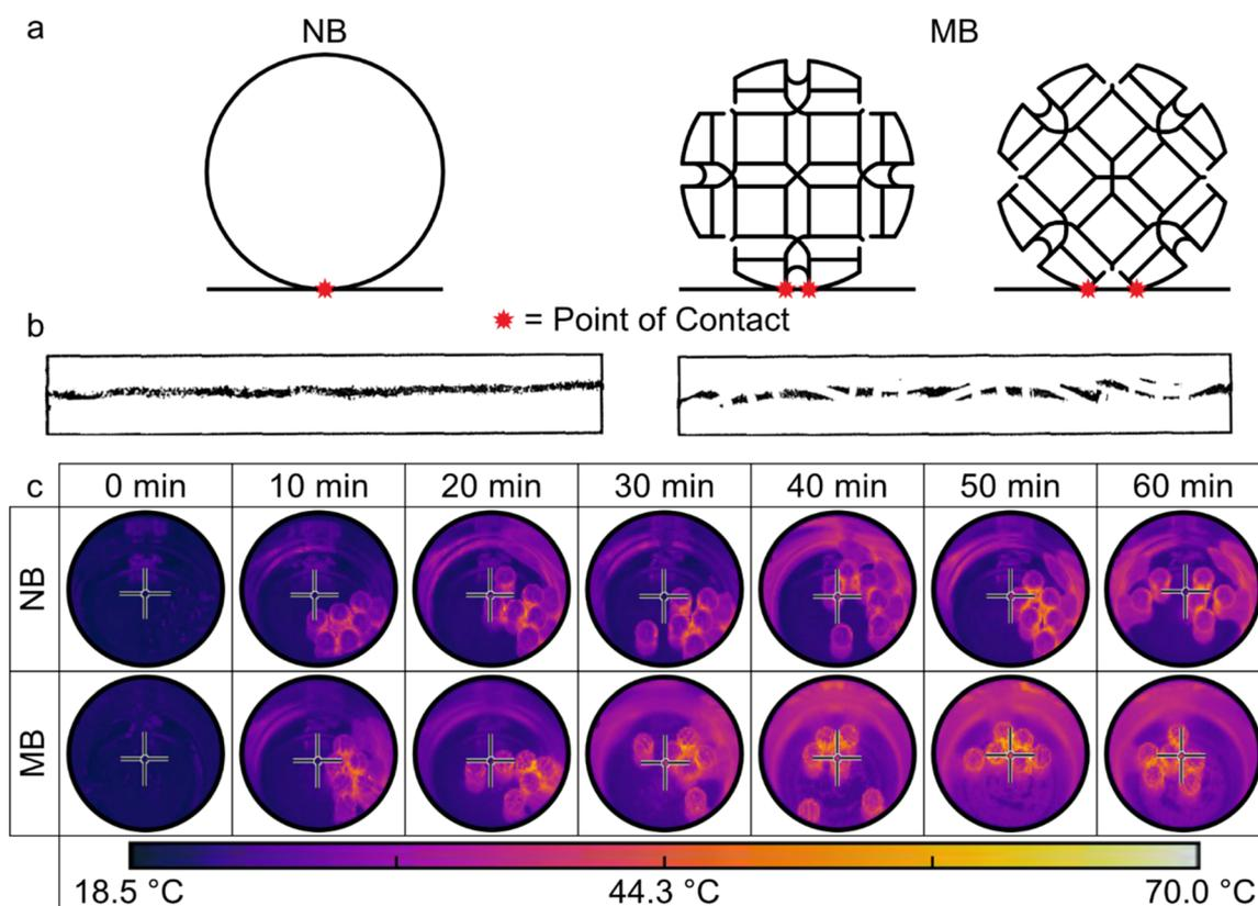
Fig. 4 (a) Possible points of contact/mechanical treatment at a given instance for both NB and MB. (b) Ink prints on paper using NB and MB showing the difference of the distribution of ball contact points. (c) Thermal images of ball-mill chamber and NB or MB after PBM captured using a FLIR camera.
