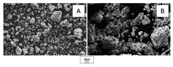
Fig. 7 SEM images of  $KCuF_3$  perovskite obtained by mechanochemical solid-state synthesis after 6 h of milling time (A) as well as by solvothermal method (B).
