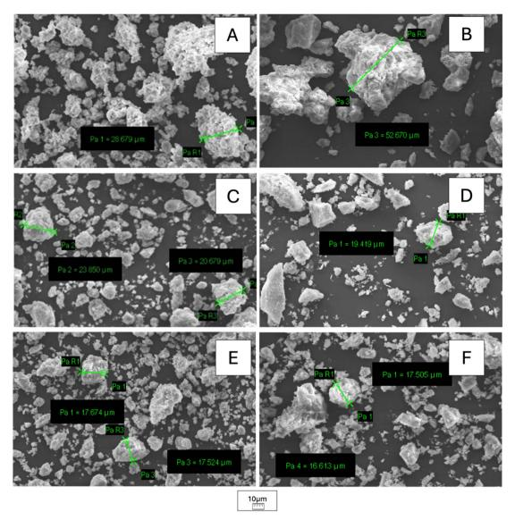
Fig. 6 SEM images of KCuF<sub>3</sub> (A-C) and KNiF<sub>3</sub> (D-F) perovskites obtained by mechanochemical solid-state synthesis at different milling times: after 3 h (A and D), 6 h (B and E) and 12 h (C and F), respectively.
