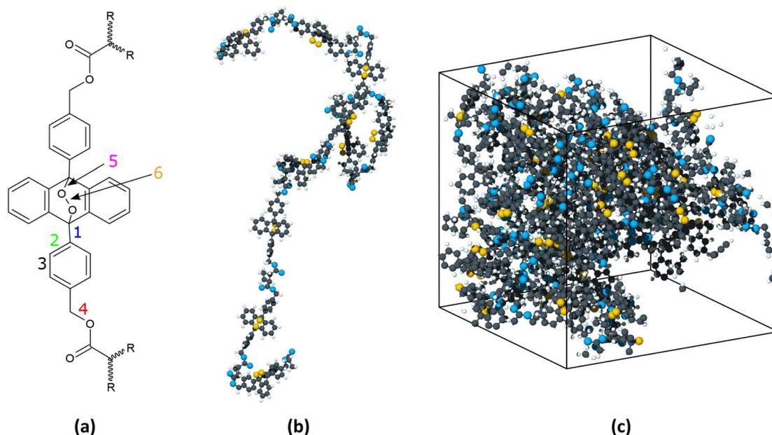
**Fig. 1** (a) Schematic of the PMA-EPO monomer where select bonds relevant to the reaction are numbered to facilitate discussion in the text. (b) Snapshot of one polymer used in the simulations. (c) Snapshot of the simulation box for the thermal reactions. The white and black spheres represent hydrogen and carbon atoms, respectively. The blue and gold spheres represent oxygen atoms, where the gold color is used to identify the atoms that will be released as oxygen molecules.
