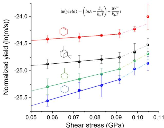
Fig. 2 Semi-log plot of the normalized yield vs. shear stress for the tribopolymers produced from cyclohexene,  $\alpha$ -pinene, methylcyclopentane, and cyclohexane vapor in  $N_2$ . The solid lines and dashed lines represent linear regression of the data points at shear stress  $\leq 0.091$  GPa and  $\geq 0.091$  GPa respectively. Error bars indicate the standard error of the mean of the reaction yield calculated from 3–4 different sliding tracks.
