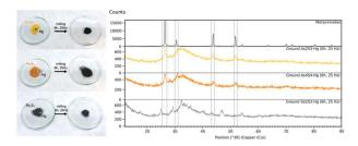
Fig. 4 Left: powders obtained upon grinding mercury with  $As_4S_4$ ,  $As_2S_3$  and  $Sb_2S_3$  respectively, from top to bottom. Right: comparison between XRPD patterns of the ground powders with that of metacinnabar (*i.e.* black HgS).
