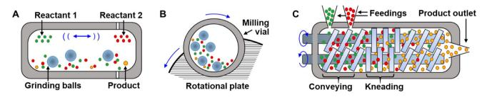
Fig. 3 Common mechanochemical reactors. (A) Ball-mill, and (B) planetary mill reactors for batch synthesis. (C) Twin-screw extruder for continuous mechanochemical production.
