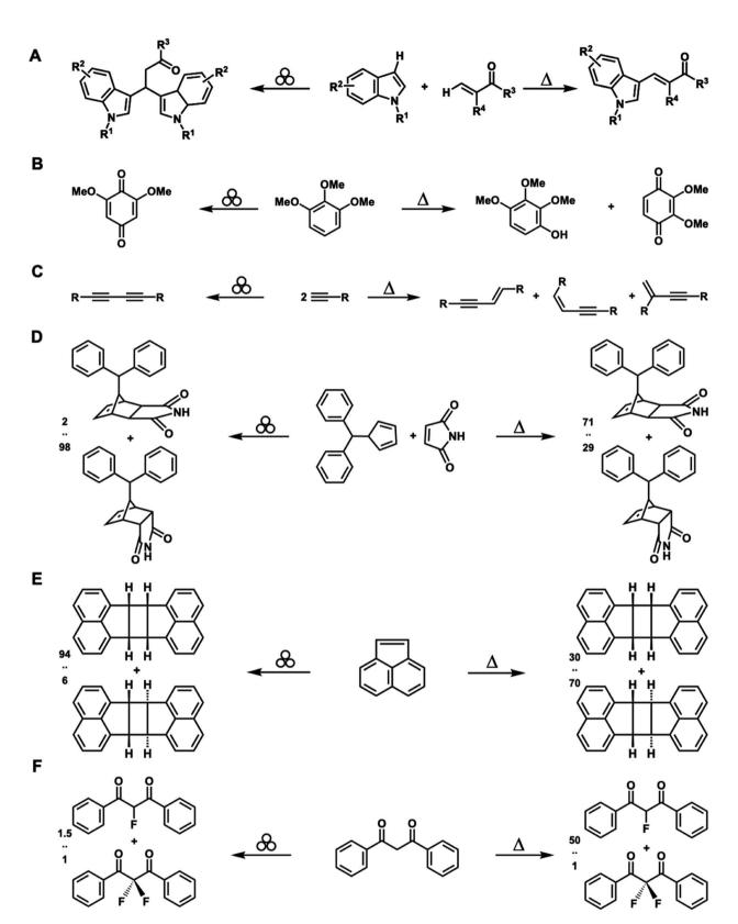
Fig. 4 Changes in selectivity under solvothermal and mechanochemical conditions. Triangles indicate solvothermal conditions, three balls indicate mechanochemical conditions. (A) Oxidative coupling of indoles with acrylates. (B) Oxidation of methoxylated aromatics. (C) Dimerization of alkynes. (D) [4 + 2] Diels-Alder reaction. (E) [2 + 2] cycloaddition reaction. (F) Fluorination of dibenzoylmethanes.
