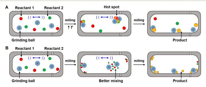
Fig. 5 Theories of mechanochemical activation. (A) Hot-spot theory: hot-spots arise as a result of collisions within mechanochemical reactors. (B) Mixing efficiency theory: increased contact between reactants as a result of increase in the surface areas of the reactants.
