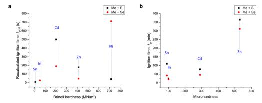
Fig. 4 Influence of hardness on the time of ignition: (a) data from this study and (b) data from (ref. 26). By T, the results from the study<sup>26</sup> are labeled. The hardness source data in our study were taken from ref. 52 and in ref. 26, it was from ref. 53 and although different types of hardness are plotted (Brinell hardness vs. microhardness), the relative differences between the metals are the same in both sources. For lead, hardness data were not available in neither of the studies
