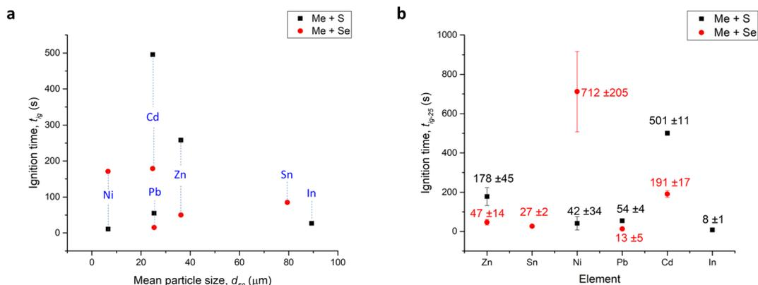
Fig. 3 (a) The dependence of  $t_{ig}$  of MSRs to yield sulfides (S) and selenides (Se) on  $d_{50}$  values and (b) re-calculated ignition time neglecting the influence of particle size and morphology ( $t_{ig-25}$ ).
