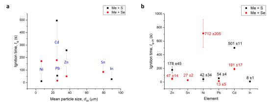
Fig. 3 (a) The dependence of  $t_{iq}$  of MSRs to yield sulfides (S) and selenides (Se) on  $d_{50}$  values and (b) re-calculated ignition time neglecting the influence of particle size and morphology ( $t_{iq-25}$ ).
