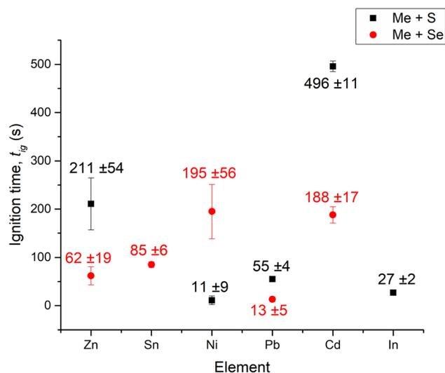
Fig. 2 Ignition times ( $t_{ig}$ ) of the investigated Me + S and Me + Se MSRs.
