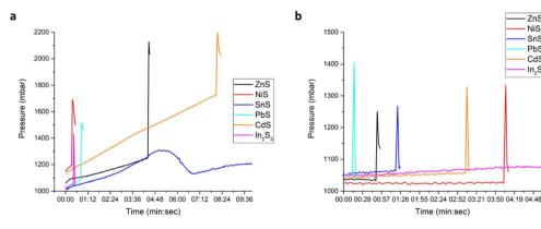
Fig. 1 Gas pressure changes during milling (representative curves): (a) Me-S mixtures treated at 750 rpm and (b) Me-Se mixtures treated at 400 rpm.
