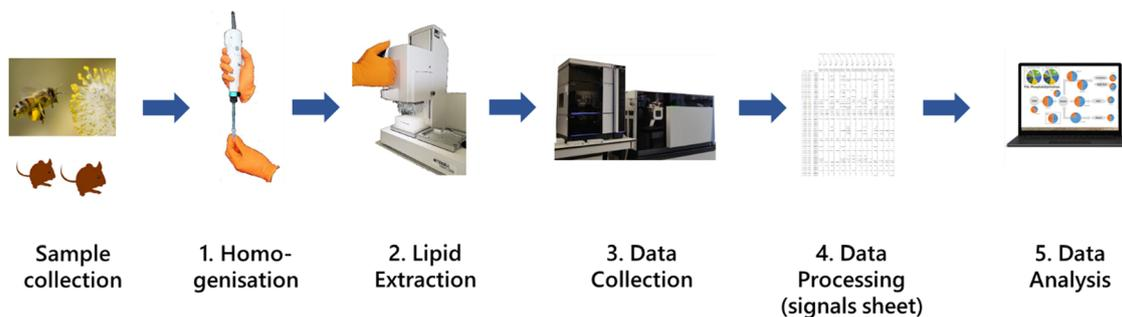
**Fig. 1** The pipeline for high throughput data collection of LCMS data from large numbers of biological samples. Samples collected from the field are stored at  $-80\text{ }^{\circ}\text{C}$  (freeze-dried if needed), then (1) homogenised, (2) the lipids extracted, (3) profiled using LCMS, (4) the data extracted and processed to give a signals sheet with metadata, and then (5) analysed.
