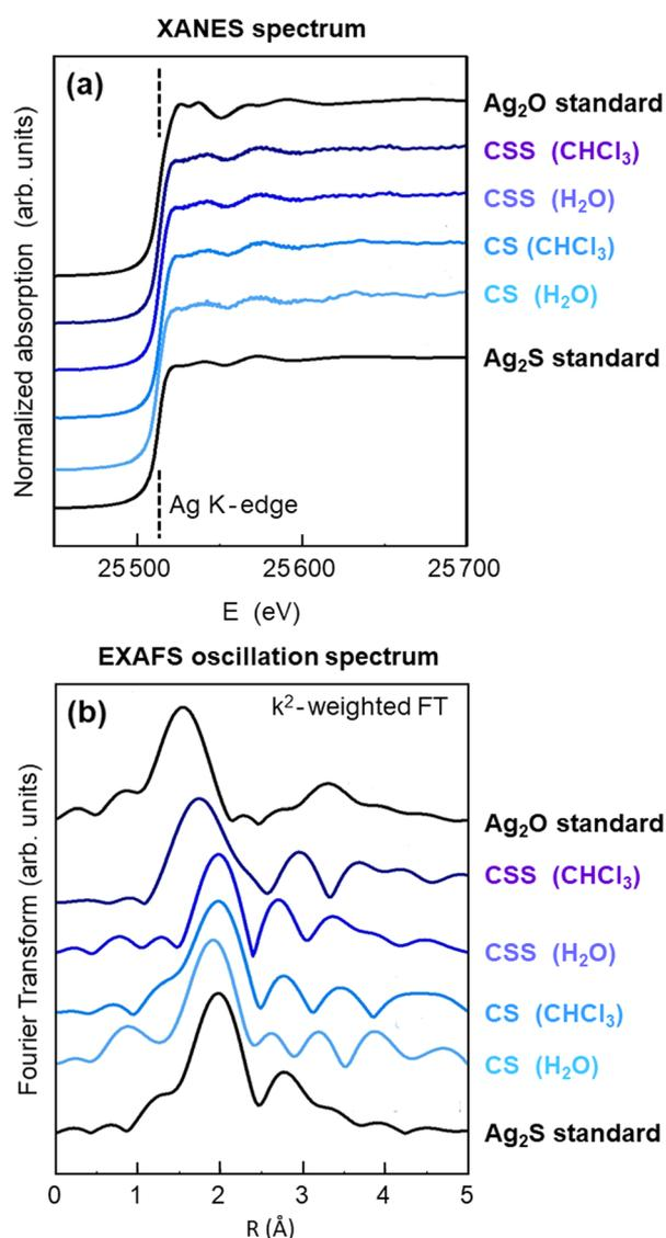
Fig. 4 (a) XANES spectra at the Ag K-edge of CS and CSS NCs solutions in CHCl<sub>3</sub> and water, compared with Ag<sub>2</sub>S and Ag<sub>2</sub>O standards. (b) Fourier transform (FT) of the  $k^2$ -weighted EXAFS oscillations, for all NCs systems shown in (a).
