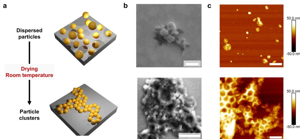
**Fig. 3** The film formation process and drying-induced aggregation of the bark-derived particulate coating. (a) Schematic illustration of the film formation process of the hybrid NPs coating. (b) SEM images demonstrating the film formation process. (c) AFM images demonstrating the film formation process (hybrid particles with 30% polyphenol). Scale bar: 400 nm.
