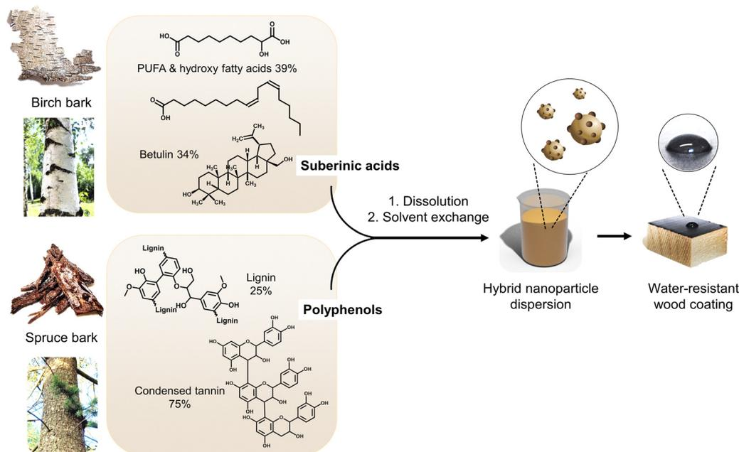
**Fig. 1** Production of bark-derived water-resistant wood coating. Birch outer bark and spruce bark were used to extract suberinic acids and polyphenols, which were then combined to form an aqueous dispersion coating. PUFA refers to polyunsaturated fatty acids.
