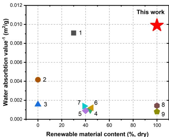
Fig. 7 Comparison of inverse of water absorption value to the biobased content of benchmark wood coating systems.<sup>40,50–54</sup> The numbers in the graph refer to the list of references in Table S1 (ESI†).
