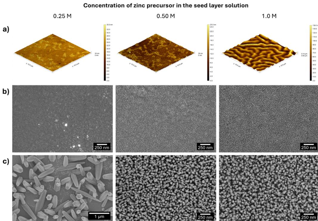
**Fig. 3** (a) AFM and (b) SEM images of the seed layers printed on PET-ITO substrates with 0.25, 0.50 and 1.0 M zinc acetate precursor solutions. (c) Morphology of the nanostructures hydrothermally grown from each seed layer.
