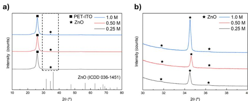
Fig. 4 XRD patterns of the (a) ZnO nanorods grown from seed layers with 0.25, 0.50 and 1.0 M precursor concentrations ( $2\theta$  between 10 and 80°). (b) Zoom of the ZnO nanorods' XRD patterns in the region between 30 and 40° ( $2\theta$ ).
