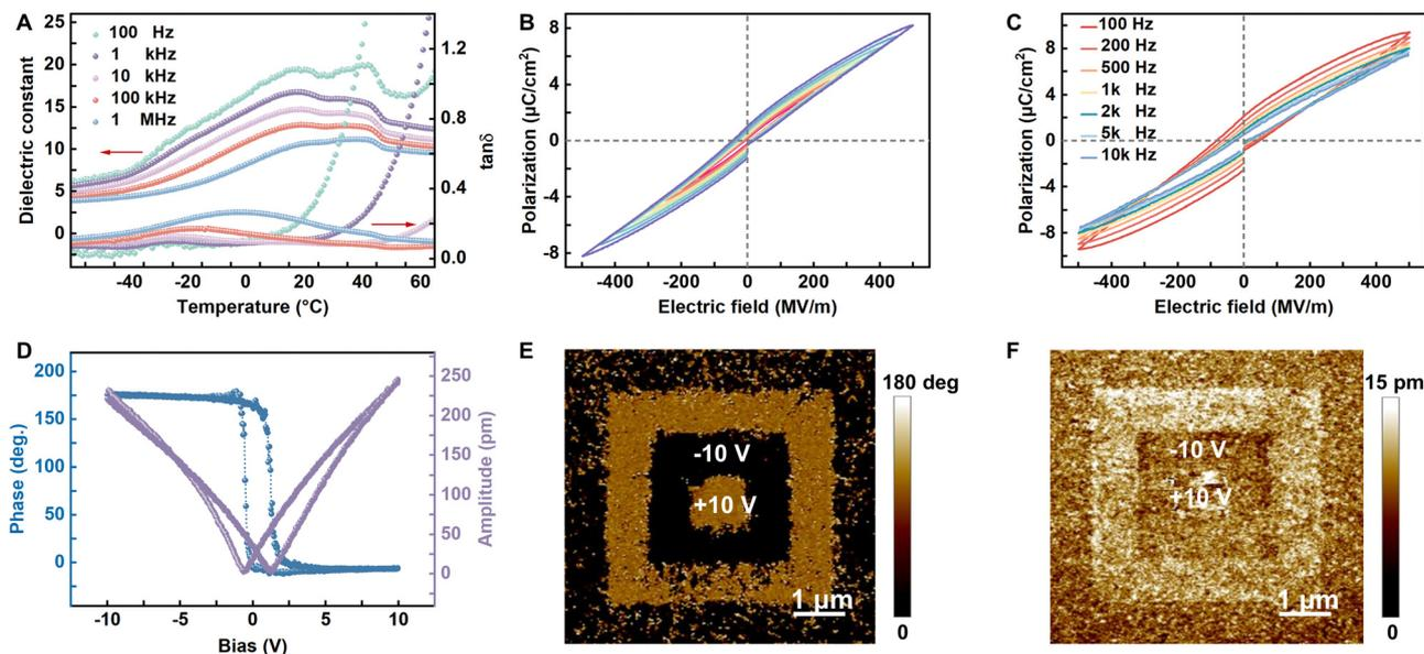
Fig. 3 Ferroelectric properties of crosslinked P(VDF-CTFE-DB) films. (A) Temperature-dependent  $\epsilon$  and dielectric loss of crosslinked P(VDF-TrFE-DB) films at different frequencies. (B), (C)  $P$ - $E$  loops of Au/C-P(VDF-CTFE-DB)/Au under varying electric fields at 1000 Hz (B) and at different frequencies (C). (D) Phase–voltage hysteresis and amplitude–voltage butterfly loop. (E), (F) Phase (E) and amplitude (F) mapping were obtained from PFM.
