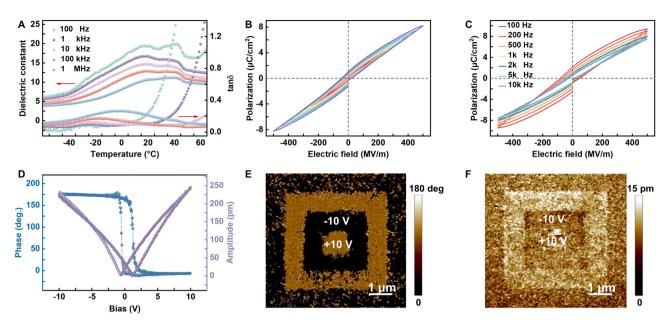
Fig. 3 Ferroelectric properties of crosslinked P(VDF-CTFE-DB) films. (A) Temperature-dependent  $\varepsilon$  and dielectric loss of crosslinked P(VDF-TrFE-DB) films at different frequencies. (B), (C) P-E loops of Au/C-P(VDF-CTFE-DB)/Au under varying electric fields at 1000 Hz (B) and at different frequencies (C). (D) Phase–voltage hysteresis and amplitude–voltage butterfly loop. (E), (F) Phase (E) and amplitude (F) mapping were obtained from PFM.
