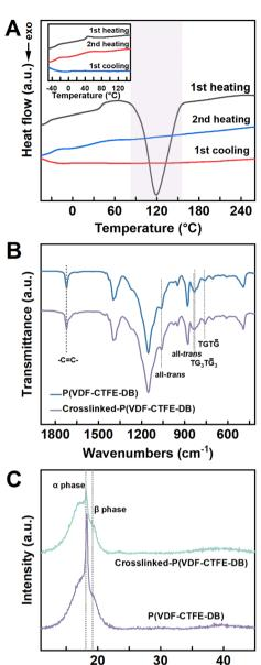
**Fig. 1** Crosslinking and crystalline properties of elastic relaxor ferroelectric films. (A) DSC curves of the blended P(VDF-CTFE-DB)/BPO/TAIC during heating and cooling cycles. (B) FT-IR spectra (C) and XRD patterns of pristine and crosslinked P(VDF-CTFE-DB).
