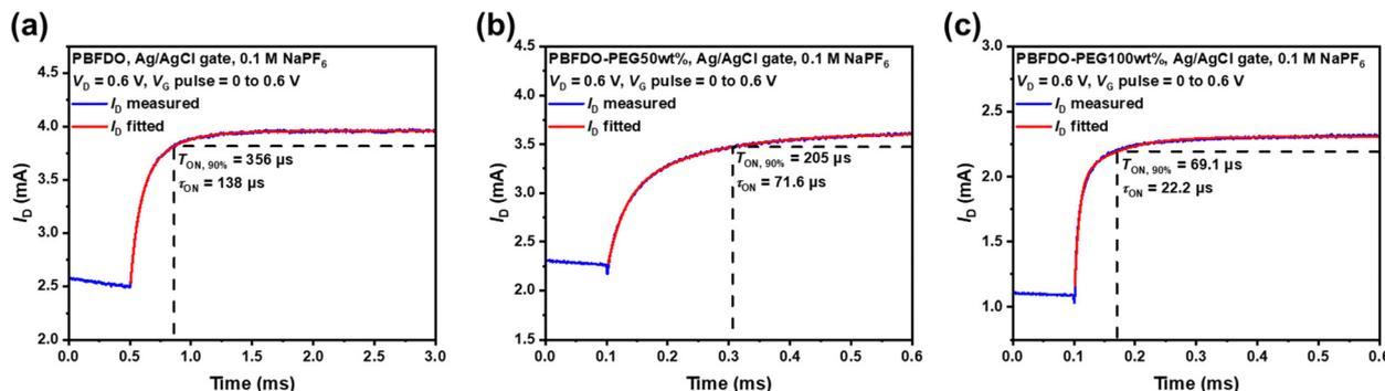
Fig. 5 Temporal response of the drain current ( $I_d$ ) of OECTs with different channel materials. (a) PBFDO; (b) PBFDO-PEG50wt%; (c) PBFDO-PEG100wt%.  $V_{gs}$  pulse amplitude = 0.6 V.  $V_G$  pulse stated from 0.5 ms (a) or 0.1 ms (b) and (c).  $T_{ON,90}$  records the time required for the  $I_D$  to grow from the beginning of  $V_G$  pulse to 90% of the increase in  $I_D$  introduced by  $V_G$  pulse.  $\tau_{ON}$  is the fitted time constant of the exponential decay curve.
