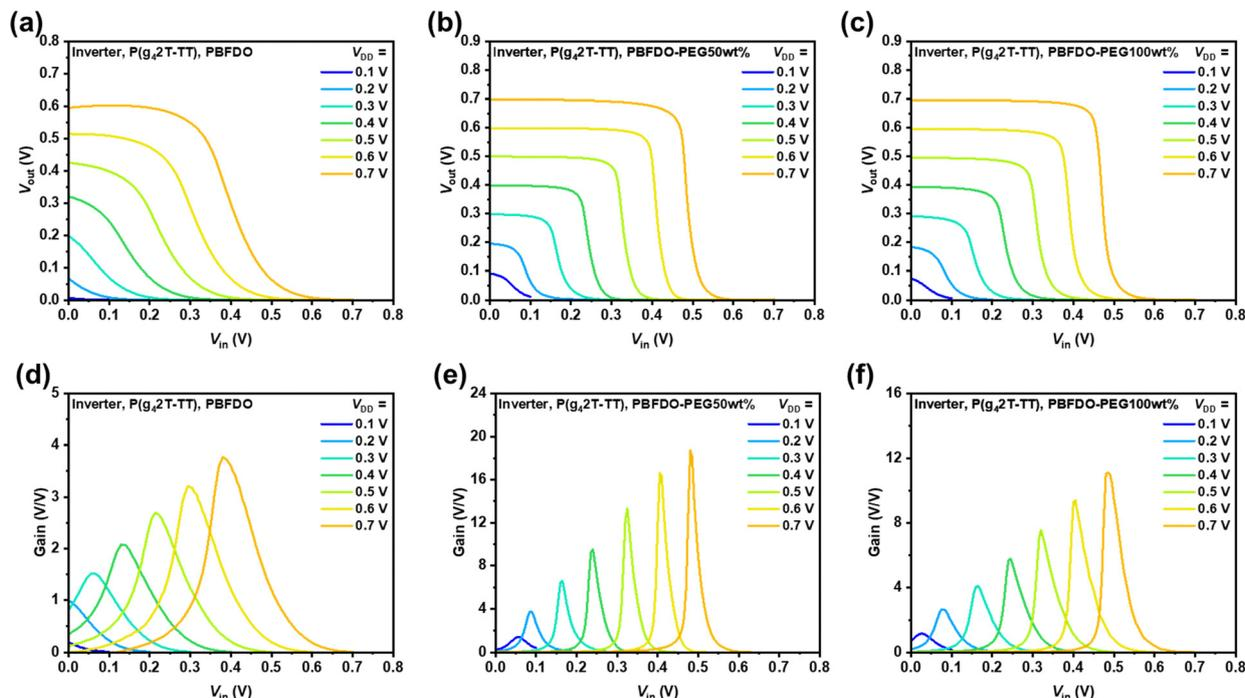
Fig. 6 OECTs-based complementary inverters. The voltage transfer characteristics and gain of inverters based on  $P(g_42T-TT)$  with different n-type channel materials (a) and (d) PBFDO, (b) and (e) PBFDO-PEG50wt%, (c) and (f) PBFDO-PEG100wt%.
