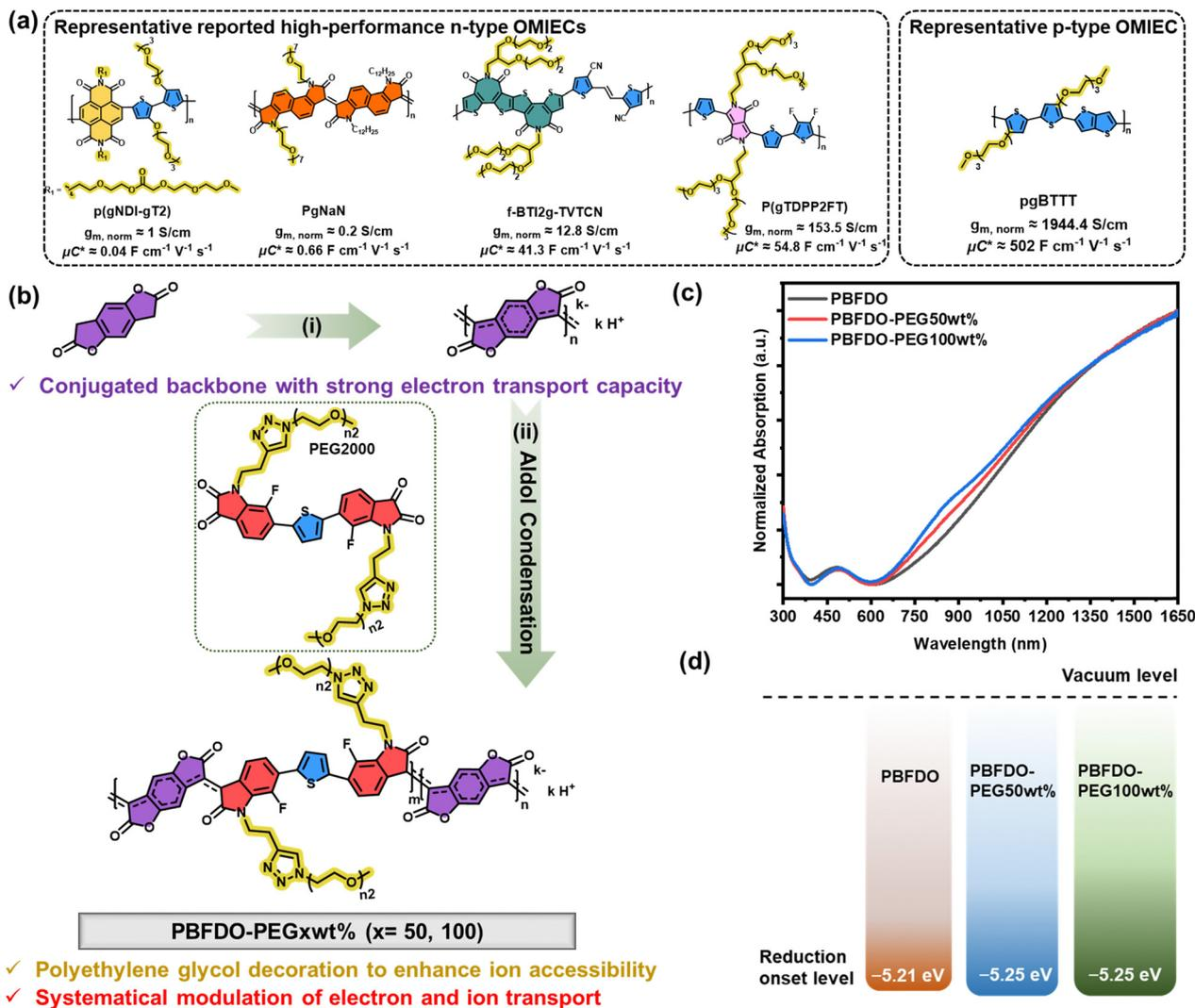
**Fig. 1** (a) The molecular structures of representative p- and n-type OMIECs. (b) Schematic illustration of synthesis of PBFDO-PEG based OMIECs. (i) TMQ, DMSO, 85 °C, 6 h and (ii) injection of PEG units, 85 °C, 8 h. (c) Optical absorption spectra of the investigated OMIECs. (d) The energy level diagram of PBFDO-PEG based OMIECs.
