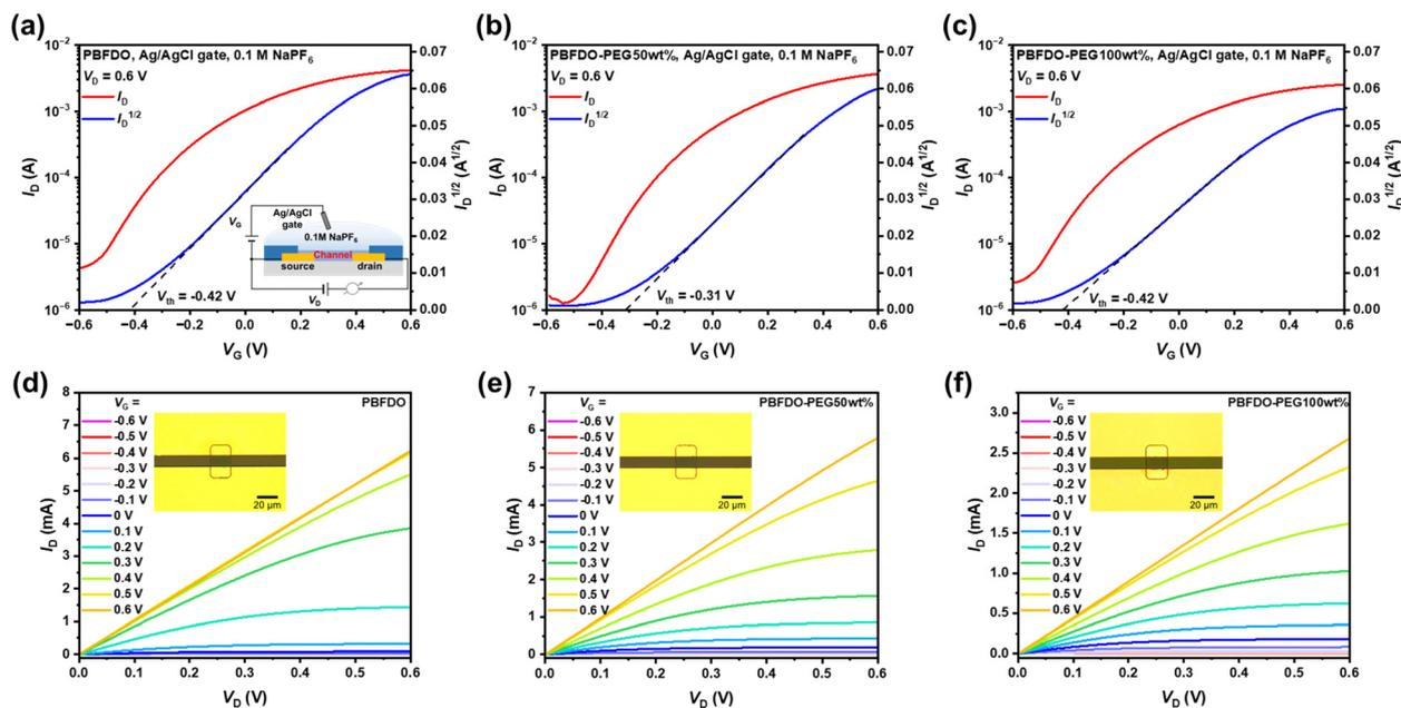
Fig. 4 Transfer (a)–(c) and output characteristics (d)–(f) of OEETs based on (a) and (d) PBFDO; (b) and (e) PBFDO-PEG50wt%; (c) and (f) PBFDO-PEG100wt%. The transfer characteristics were measured at  $V_{ds} = 0.6$  V. The channel dimension used for this measurement is channel width/length =  $20 \mu\text{m}/10 \mu\text{m}$ , while the thickness was around  $70$  nm. Inset: Illustration of the OEET structure (a) and optical microscopic photos of the corresponding OEET channels (d)–(f).
