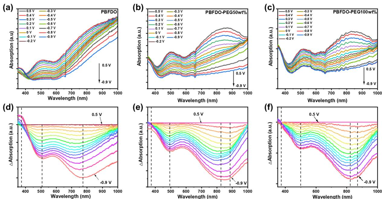
Fig. 3 Potential dependent UV-vis absorption spectra of the PBFDO-PEG/ITO electrode measured in 0.1 M NaPF<sub>6</sub> aqueous solution with Ag/AgCl as the reference electrode. (a)–(c) *In situ* UV-vis absorption spectra of PBFDO, PBFDO-PEG50wt% and PBFDO-PEG100wt%. (d)–(f) Corresponding differential absorption spectra at select voltages during CV scan.
