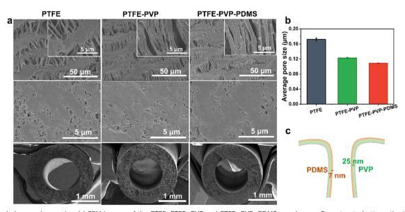
Fig. 2 Morphology and pore size. (a) SEM images of the PTFE, PTFE-PVP and PTFE-PVP-PDMS membranes. From top to bottom, the inner cavity surface, outer wall surface, and cross section morphology of the hollow fiber. (b) Average pore size. (c) Thickness of the PVP hydrogel layer and PDMS slippery layer was calculated by the pore size.
