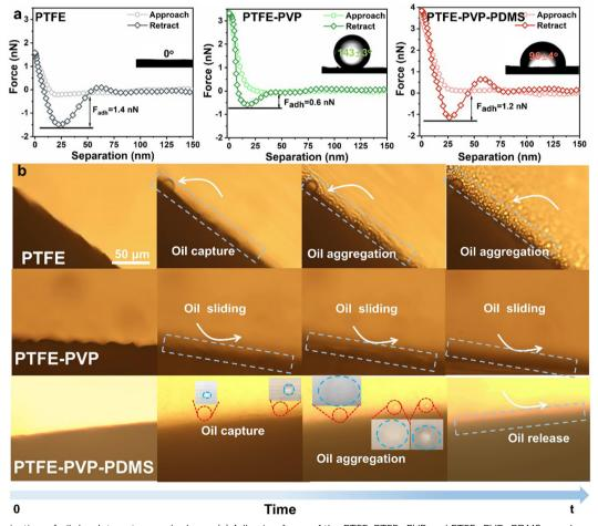
Fig. 4 Characterization of oil droplet capture and release. (a) Adhesion force of the PTFE, PTFE-PVP and PTFE-PVP-PDMS membrane to oil using the AFM test. The inset image shows the contact angle of underwater oil for the corresponding membrane. The movement of oil droplets in an emulsion on the surface of (b) PTFE, (c) PTFE-PVP, and (d) PTFE-PVP-PDMS membrane. The gray inset shows an oil droplet at 4× magnification.
