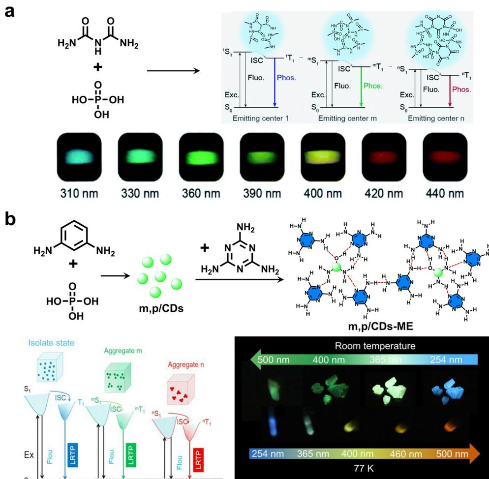
**Fig. 10** (a) The preparation of excitation-dependent multicolor CD RTP materials by a one-pot hydrothermal synthesis of biuret and phosphoric acid. Reproduced with permission from ref. 79. Copyright 2022, Royal Society of Chemistry. (b) The synthesis of green-light-excitable CD crystals (m,p/CDs-ME) that exhibited excitation-dependent RTP emission. Reproduced with permission from ref. 80. Copyright 2022, American Chemical Society.
