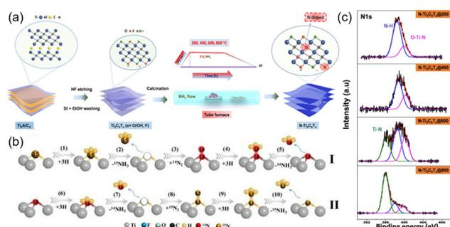
Fig. 5 (a) Illustration of synthesis of N-doped MXene from the  $\text{Ti}_3\text{AlC}_2$  MAX phase.<sup>62</sup> Copyright 2019, American Chemical Society. (b) The proposed N dopants in 15N doped- $\text{TiV-Ti}_{3-x}\text{C}_2\text{Ty-1.2}$  MXene catalysts act as an active catalytic site in ENRR.<sup>63</sup> Copyright 2021, Elsevier. (c) Core-level XPS of the N 1s of N-doped MXene samples annealed at various temperatures.<sup>63</sup> Copyright 2021, Elsevier.
