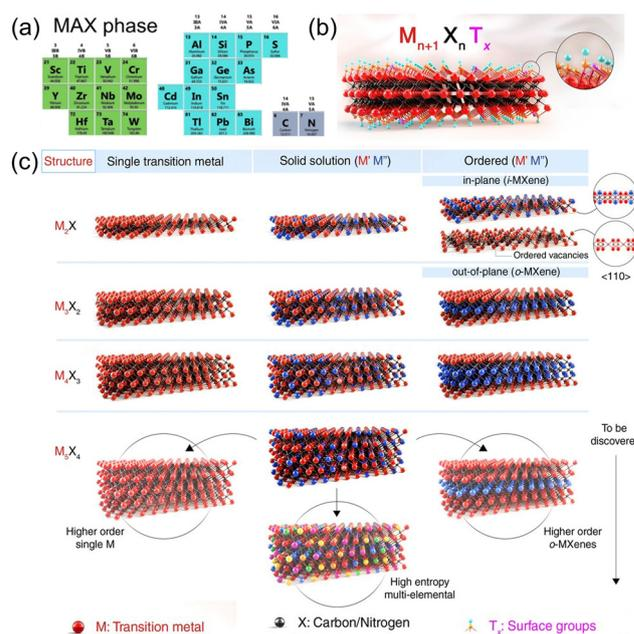
Fig. 2 (a) Composition of various types of MAX.<sup>30</sup> Copyright 2023, Elsevier. (b) and (c) Schematic illustration of the MXene structures.<sup>29</sup> Copyright 2021, AAAS.
