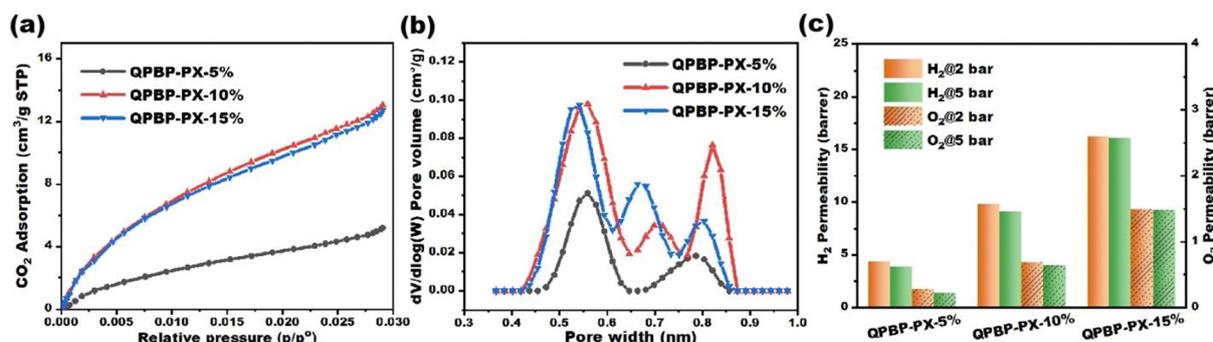
Fig. 2 (a) CO<sub>2</sub> adsorption isotherms, (b) pore size distributions, and (c) H<sub>2</sub> and O<sub>2</sub> permeabilities of QBPB-PX-5%, QBPB-PX-10%, and QBPB-PX-15%.
