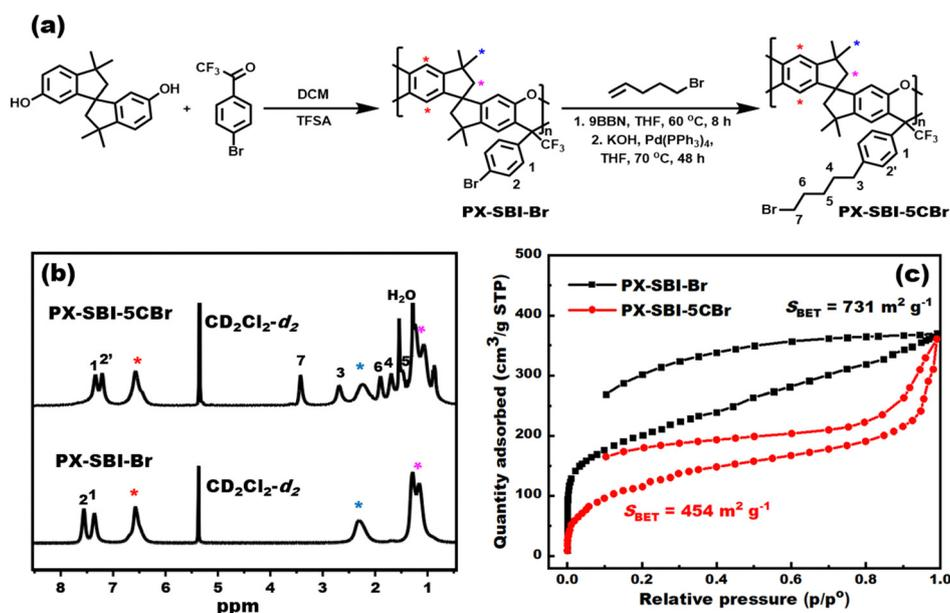
Fig. 1 (a) Synthetic route, (b) <sup>1</sup>H NMR spectra, and (c) N<sub>2</sub> adsorption/desorption isotherms of PX-SBI-Br and PX-SBI-5CBBr.
