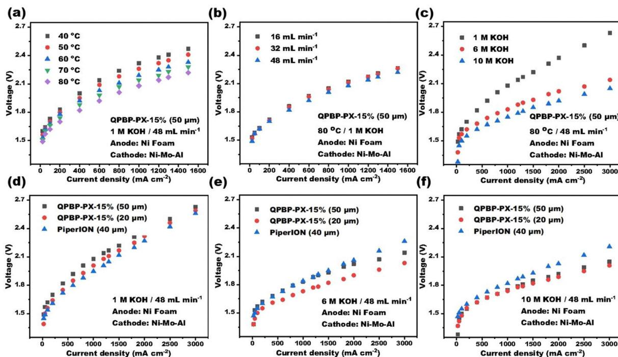
Fig. 6 *I*-*V* polarization curves of QBPB-PX-15% based AEMWE with varying (a) temperatures, (b) flow rates of circulating alkaline solution, and (c) concentrations of KOH solution; *I*-*V* polarization curves of AEMWEs based on QBPB-PX-15% (50  $\mu\text{m}$ ), QBPB-PX-15% (20  $\mu\text{m}$ ), and PiperION (50  $\mu\text{m}$ ) in (d) 1 M, (e) 6 M, and (f) 10 M KOH solutions at a cell temperature of 80 °C and flow rate of 48 mL  $\text{min}^{-1}$ .
