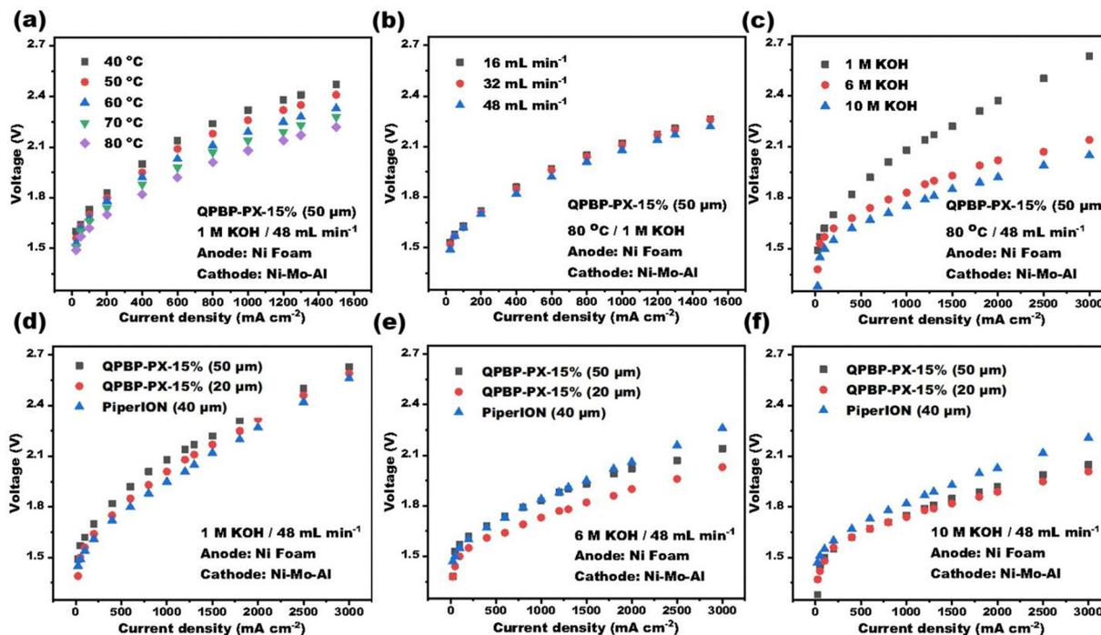
Fig. 6 *I*-*V* polarization curves of QBPB-PX-15% based AEMWE with varying (a) temperatures, (b) flow rates of circulating alkaline solution, and (c) concentrations of KOH solution; *I*-*V* polarization curves of AEMWEs based on QBPB-PX-15% (50 μm), QBPB-PX-15% (20 μm), and PiperION (50 μm) in (d) 1 M, (e) 6 M, and (f) 10 M KOH solutions at a cell temperature of 80 °C and flow rate of 48 mL min<sup>-1</sup>.
