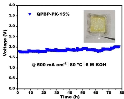
Fig. 7 Durability of QBPB-PX-15% based AEMWE at 80 °C, 500 mA cm<sup>-2</sup>, and in 6 M KOH solution.
