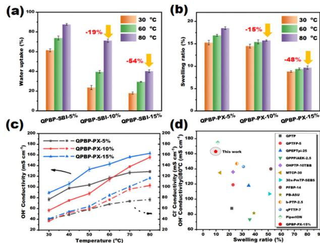
Fig. 4 (a) WU and (b) SR of QBPB-PX-*x* at 30, 60, and 80 °C. (c) Temperature dependence of OH<sup>−</sup> and Cl<sup>−</sup> conductivities of QBPB-PX-5%, QBPB-PX-10%, and QBPB-PX-15%. (d) Comparison of QBPB-PX-15% with commercial PiperION and earlier reported poly(aryl piperidinium) AEMs.<sup>20,27,33,35,38–41</sup>
