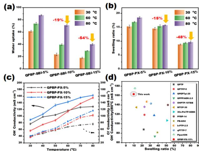
Fig. 4 (a) WU and (b) SR of QBPB-PX-*x* at 30, 60, and 80 °C. (c) Temperature dependence of OH<sup>−</sup> and Cl<sup>−</sup> conductivities of QBPB-PX-5%, QBPB-PX-10%, and QBPB-PX-15%. (d) Comparison of QBPB-PX-15% with commercial PiperION and earlier reported poly(aryl piperidinium) AEMs.<sup>20,27,33,35,38–41</sup>
