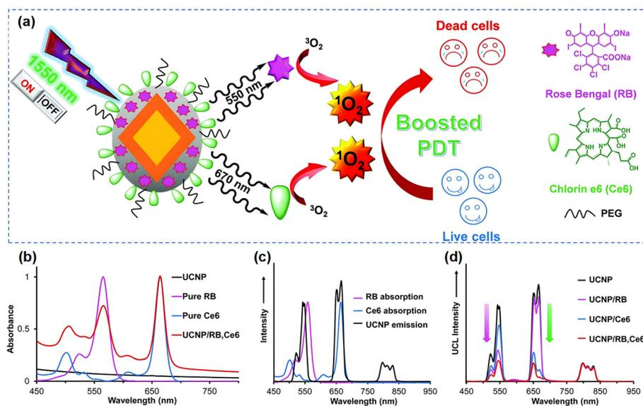
Fig. 8 (a) Schematic diagram of the formation of UCNP@SiO<sub>2</sub>/RB,Ce<sub>6</sub>. (b) The absorbance of UCNP, RB, Ce<sub>6</sub>, UCNP/RB,Ce<sub>6</sub>. (c) The absorption and emission spectra of RB, Ce<sub>6</sub> and UCNP respectively. (d) The UCL spectra of UCNP, UCNP/RB, UCNP/Ce<sub>6</sub> and UCNP/RB,Ce<sub>6</sub> under irradiation at 1550 nm. Reproduced with permission from ref. 58. Copyright 2014, The Royal Society of Chemistry.
