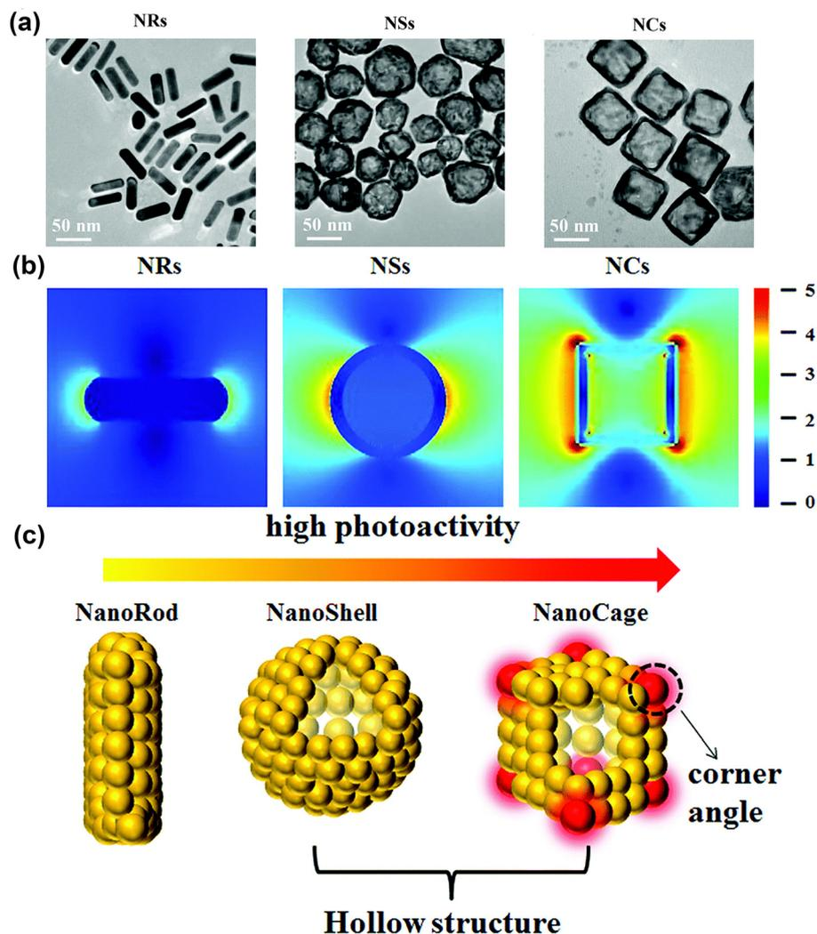
Fig. 4 (a) TEM images of Au NRs, NSs and NCs. (b) The electric field distribution and enhancement ( $|E|/|E_0|$ ) contours of Au NRs, NSs and NCs. (c) Illustration of the photoactivity of Au nanostructures. Reproduced with permission from ref. 103. Copyright 2018, The Royal Society of Chemistry.
