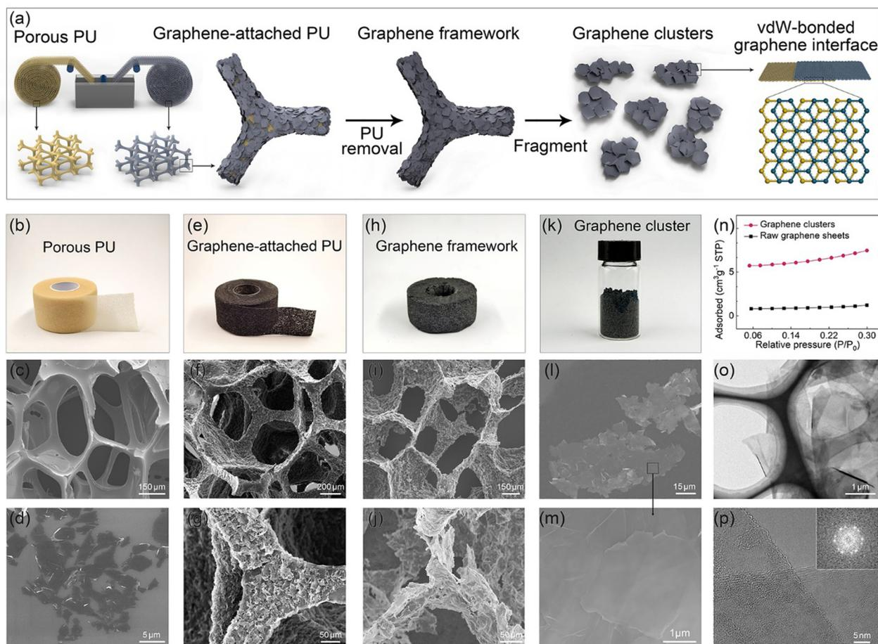
**Fig. 1** (a) Schematic illustrating the preparation of graphene clusters. (b) Optical and (c) SEM images of the porous PU film. (d) Typical SEM image of the raw graphene sheets. Optical and SEM images of (e)–(g) graphene-attached PU, (h)–(j) graphene framework and (k)–(m) graphene clusters. (n)  $N_2$  isothermal sorption curves of raw graphene sheets and graphene clusters. (o) and (p) Typical TEM images and the selected area electric diffraction patterns (SAED) of graphene clusters.
