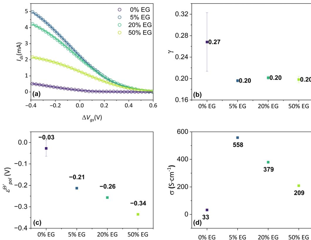
Fig. 6 (a) Transfer curves (hollow circles) from Rivnay (2016), and fitting curves (solid lines), (b)  $\gamma$ , (c)  $E_{pol}^{el}$  and (d)  $\sigma$  parameters. Reprinted (adapted) with permission from Rivnay *et al.* (2016).<sup>47</sup> For all adjustments  $R^2 = 0.99$  and  $p$ -values  $< 0.05$ .
