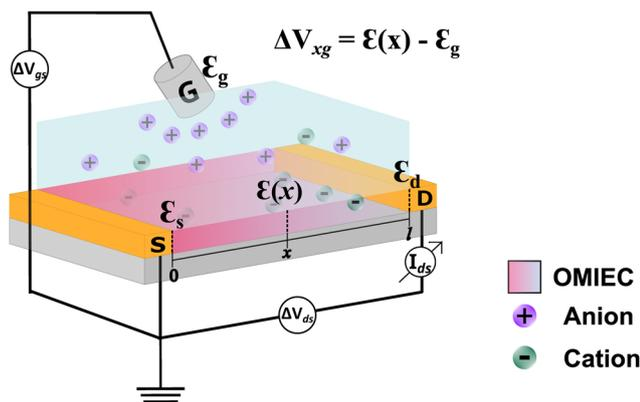
Fig. 1 Schematic representation of a typical OEET structure.
