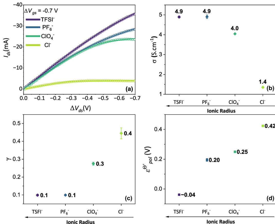
Fig. 5 (a) Output curves (hollow circles) from Flagg (2018), and fitting curves (solid lines) (b)  $\sigma$ , (c)  $\gamma$  and (d)  $\epsilon_{pol}^{\theta}$  parameters. Reprinted (adapted) with permission from Flagg *et al.* (2018).<sup>26</sup> Copyright © 2018, American Chemical Society. All data fittings with  $R^2 = 0.99$  and  $p$ -values  $< 0.05$ .
