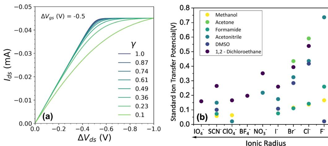
Fig. 4 (a) Effect of  $\gamma$  variation on output curve shape. Here were used the following parameters  $w = 1.5$  mm,  $h = 100$  nm,  $l = 250$   $\mu\text{m}$ ,  $\sigma = 1.5$  S  $\text{cm}^{-1}$ ,  $\sigma_{\text{res}} = 1 \times 10^{-4}$  S  $\text{cm}^{-1}$ ,  $\mathcal{E}_{\text{pol}}^{\text{el}} = 0$  V,  $T = 298.15$  K,  $\Delta V_{\text{gs}} = -0.5$  V. (b) Standard Ion Transfer Potential for anions from water to organic solvent from ref. 66–68 with adaptations.
