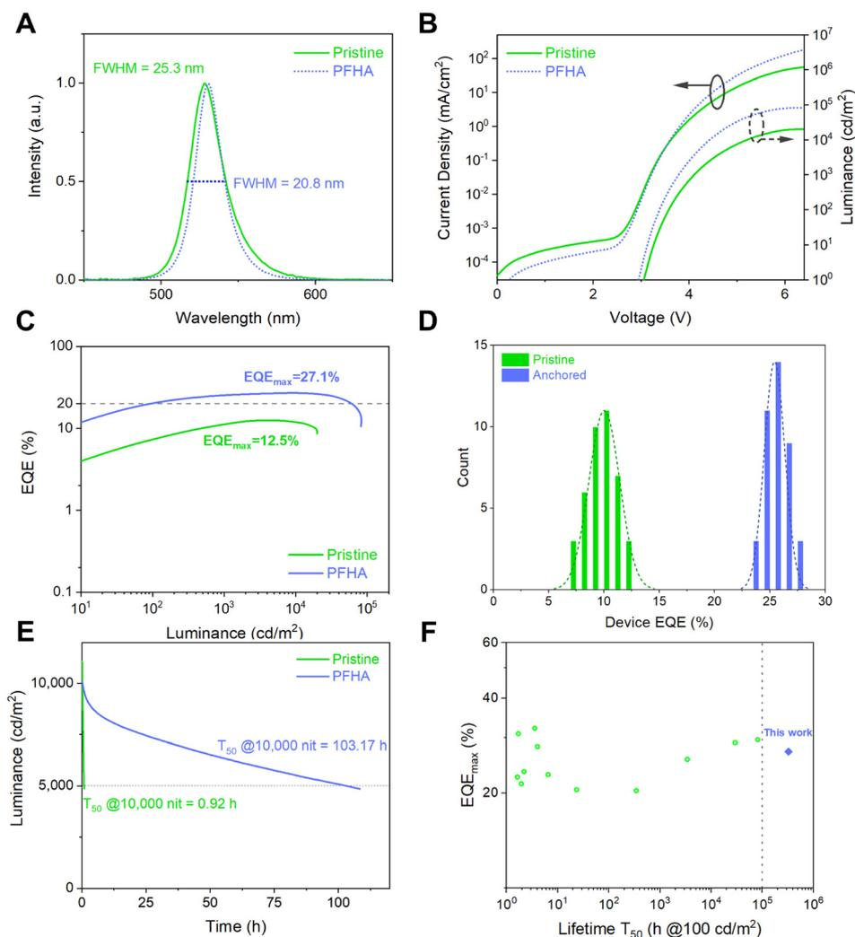
**Fig. 4** Ultra-stable and efficient PeLEDs. (A) EL spectra and (B)  $J$ – $V$ – $L$  plots of a representative PeLED device. (C) EQE to luminance curve of PeLEDs. (D) Statistical device EQE<sub>max</sub> of pristine and PFHA PeLEDs. 40 devices are measured in total. (E) Operational lifetime of pristine and PFHA-anchored PeLED devices. (F) Summary of the reported PeLED performance based on the maximum EQE and estimated or measured  $T_{50}$  at 100 cd m<sup>-2</sup>.
