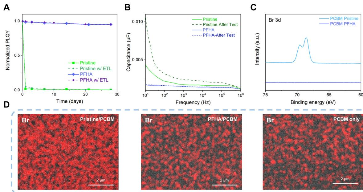
**Fig. 3** Phase stabilization and ion immobilization. (A) PLQY change with time for pristine and anchored perovskite films in ambient air. (B) Capacitance to frequency results of pristine and PFHA anchored PeLED devices. (C) Surface XPS spectra of the PCBM surface of pristine and PFHA devices. (D) SEM-EDX mapping results of the Br element on the PCBM surfaces of pristine, PFHA anchored samples and PCBM only samples.
