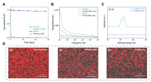
Fig. 3 Phase stabilization and ion immobilization. (A) PLQY change with time for pristine and anchored perovskite films in ambient air. (B) Capacitance to frequency results of pristine and PFHA anchored PeLED devices. (C) Surface XPS spectra of the PCBM surface of pristine and PFHA devices. (D) SEM-EDX mapping results of the Br element on the PCBM surfaces of pristine, PFHA anchored samples and PCBM only samples.
