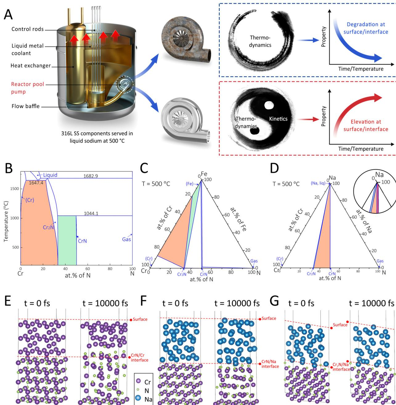
**Fig. 1** (A) Illustration of the proposed interface-engineering strategy for developing a self-organized sandwich coating structure with enhanced properties for sodium-cooled fast reactors (SFRs). (B) Cr–N binary phase diagram. (C) Isothermal section of the Cr–Fe–N system at 500 °C. (D) Isothermal section of the Cr–Na–N system at 500 °C. *Ab initio* molecular dynamics (AIMD) results of (E) CrN/Cr, (F) CrN/Na, and (G) Cr<sub>2</sub>N/Na interface structures simulated at 500 °C for 10 000 fs.
