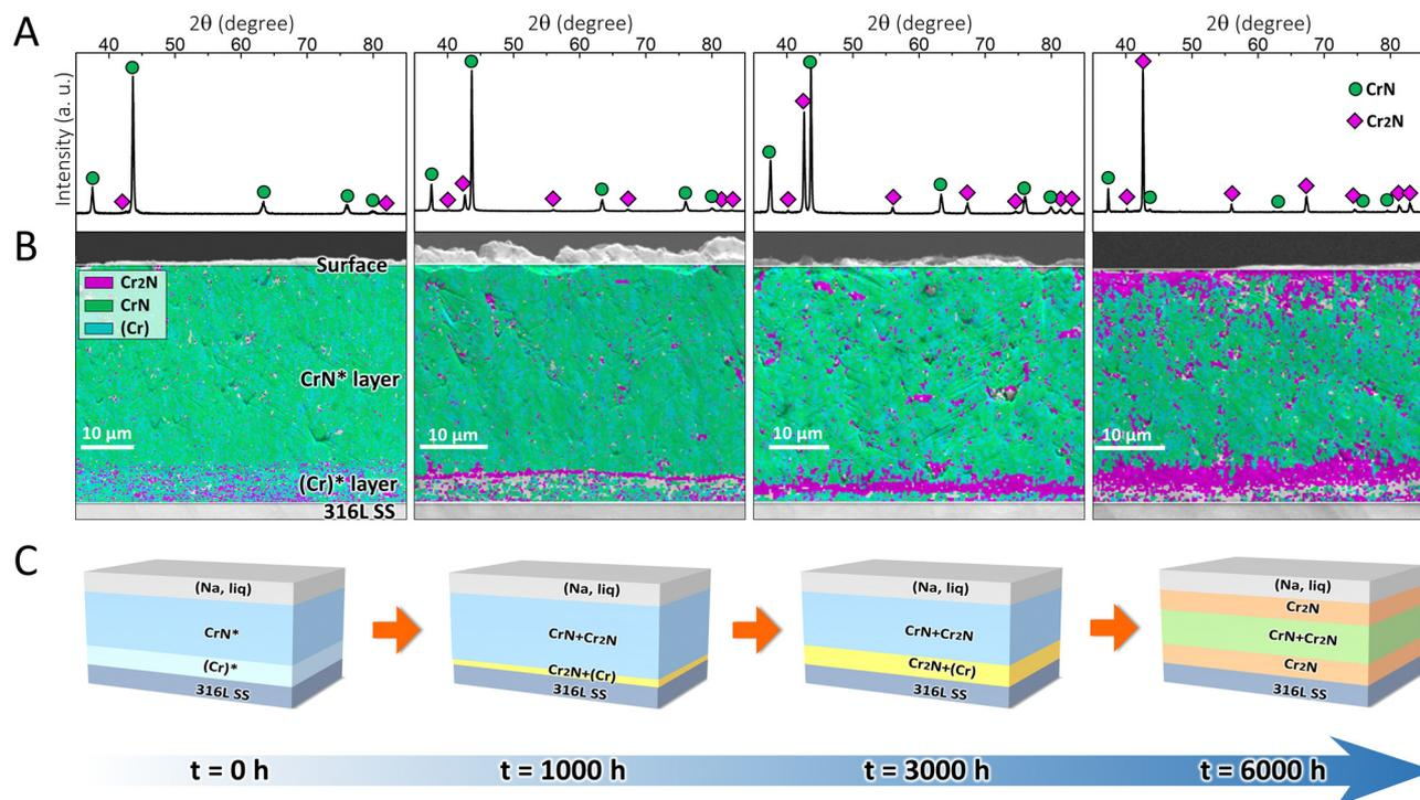
Fig. 2 (A) X-ray diffraction (XRD) patterns and (B) electron backscatter diffraction (EBSD) phase maps of the as-deposited CrN\*/(Cr)\* coating and the coating immersed in liquid sodium at 500 °C for 1000, 3000, and 6000 h. (C) Schematic diagrams of the stepwise formation of a self-organized sandwich structure composed of Cr<sub>2</sub>N/CrN/Cr<sub>2</sub>N. The asterisk denotes the main phase in each layer.
