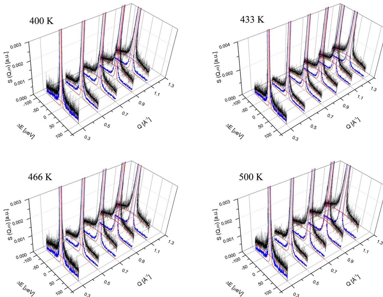
Fig. 9  $S(Q, \omega)$  of  $\text{La}_{0.8}\text{Ba}_{1.2}\text{GaO}_{3.9}$  at 400, 433, 466, and 500 K. The open circles represent the experimental data. The fit comprises of the elastic peak (blue line) and the two QE components (red lines).<sup>355</sup> Reprinted with permission from (*Chem. Mater.*, 2013, **25**, 2741–2748). Copyright (2020) American Chemical Society.
