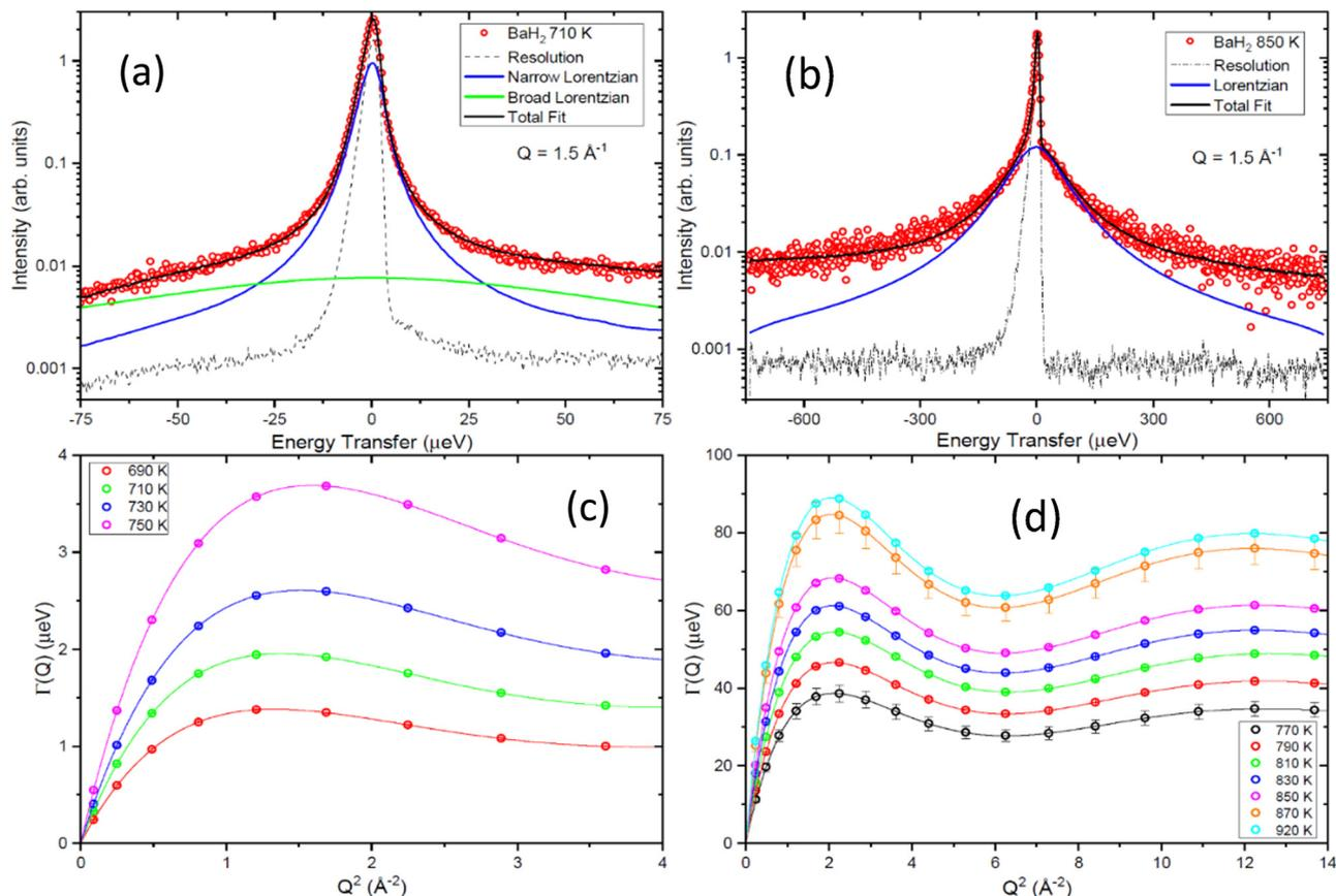
Fig. 8 The QENS measured for BaH<sub>2</sub> at BASIS (a) at  $T = 710$  K, and (b) at  $T = 850$  K. (c) and (d) show the HWHM at measured temperatures modeled with the Chudley-Elliott model. Reprinted with permission from<sup>334</sup> (*Sci. Rep.*, 2022, **12**, 6194).
