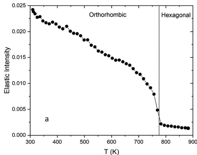
Fig. 7 Elastic intensity as a function of temperature from  $\text{BaH}_2$  measured at BASIS. Reprinted with permission from<sup>334</sup> (*Sci. Rep.*, 2022, **12**, 6194).
