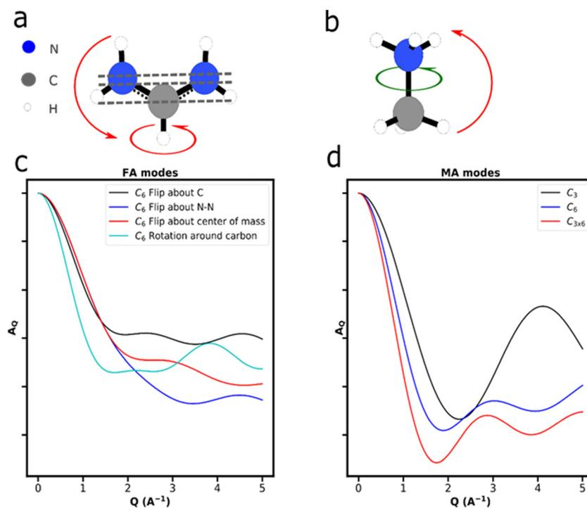
**Fig. 10** The possible rotations of (a) FA and (b) MA molecules. The green arrow indicates a  $C_3$  rotation. The red arrows indicate a  $C_6$  rotation. The grey dashed line shows the possible centers for the  $C_6$  rotation of the FA molecule. EISF models for (c) FA and (d) MA. Reprinted with permission from (ACS Nano, 2020, **14**, 15107–15118). Copyright (2020) American Chemical Society.
