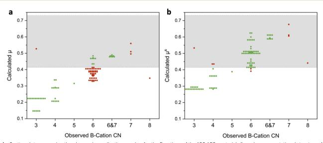
Fig. 1 Scatter plots comparing the observed coordination number for the B-cations of the 100 ABS, materials (based on computational structures from Materials Project) compared to the calculated octahedral factor based on (a) oxide derived radii and (b) sulfide derived radii. Correct predictions are marked with a green circle and incorrect predictions are marked with a red circle
