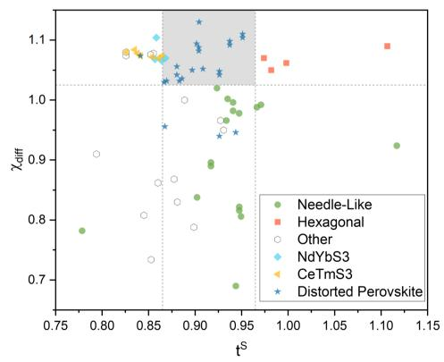
Fig. 2 Scatter plot for the 67 materials that passed the modified octahedral factor screening comparing their calculated tolerance factor, t<sup>S</sup> and their electronegativity difference,  $\chi_{diff}$ , and sorted by their crystal structure.
