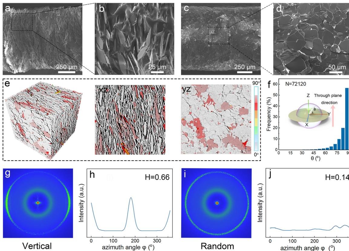
**Fig. 2** (a) and (b) SEM images of Pad-75-V from XZ view. (c) and (d) SEM images of Pad-75-V from YZ view. (e) Reconstructed model with angle distribution of micro-CT result of Pad-75-V. (f) Statistical analysis of angle distribution of BN. (g)–(j) WAXD patterns, azimuth angle curves and Herman's orientation parameters of Pad-75-V and Pad-75-R.
