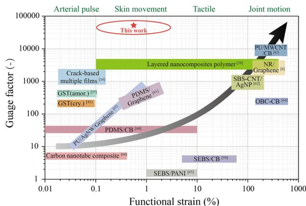
Fig. 6 A comparison of gauge factor and functional strain with other materials.
