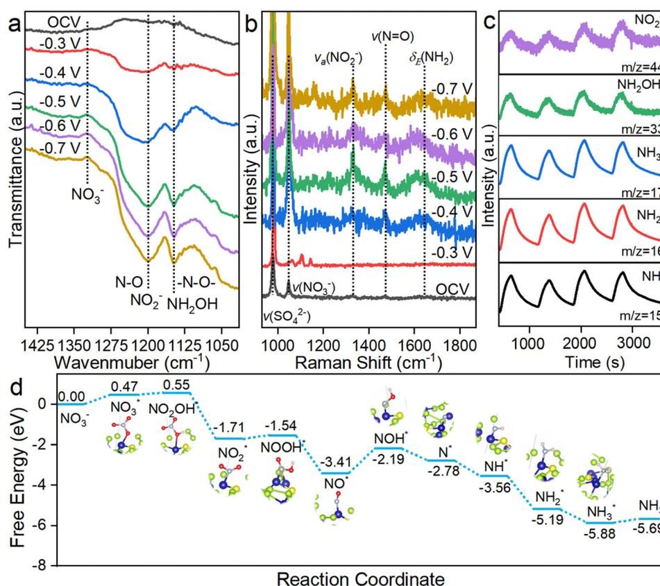
Fig. 4 (a) Electrochemical *in situ* FTIR spectra and (b) *in situ* Raman spectra of  $\text{S-CoSe}_2$  NWs. (c) Online DEMS of  $\text{S-CoSe}_2$  NWs under a potential of  $-0.35\text{ V}$  vs. RHE. (d) Reaction-free energies for different intermediates of NARR based on the model of sulfur-doped  $\text{CoSe}_2$ .
