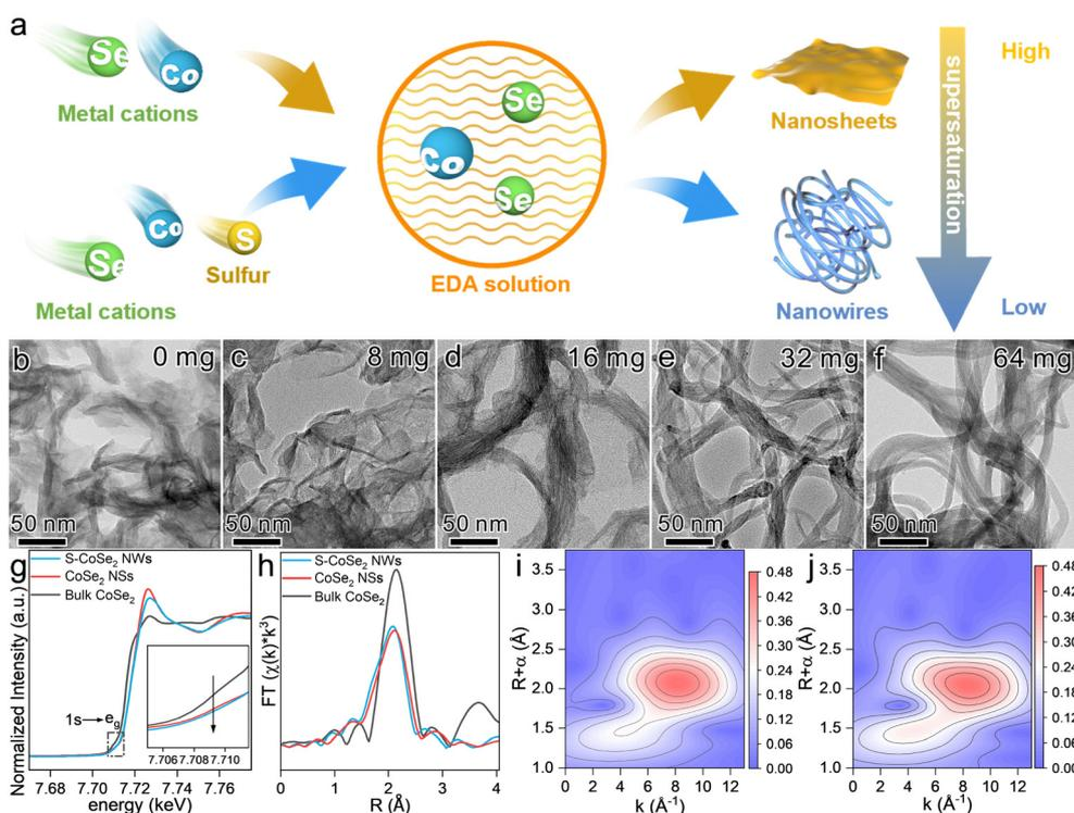
Fig. 2 (a) Formation mechanism of  $\text{CoSe}_2$  NSs and S- $\text{CoSe}_2$  NWs. (b)–(f) Morphological evolution of  $\text{CoSe}_2$  materials with different sulfur contents. (g) Co K-edge XANES spectra and (h) corresponding Fourier transforms of  $k^3$ -weighted EXAFS spectra for  $\text{CoSe}_2$  materials. Wavelet transforms of  $k^3$ -weighted EXAFS spectra of the Co K-edge for (i)  $\text{CoSe}_2$  NSs and (j) S- $\text{CoSe}_2$  NWs.
