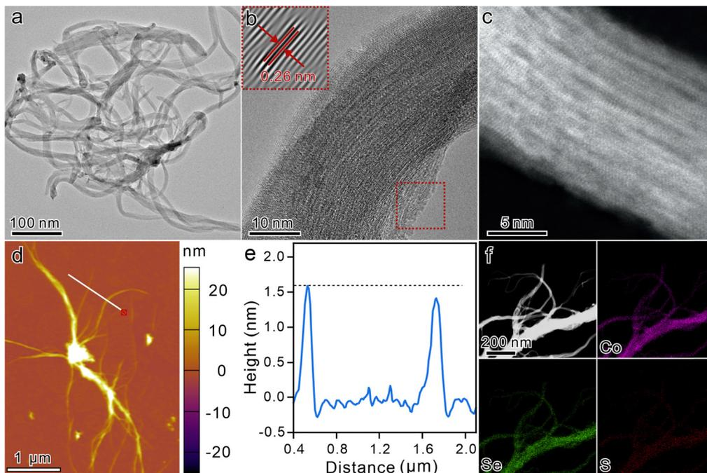
**Fig. 1** Microstructure characterization of S-CoSe<sub>2</sub> NWs: (a) TEM image; (b) HRTEM image (inset image shows the lattice fringe spacing); (c) AC HAAD-STEM image; (d) and (e) AFM image and the corresponding height profile; and (f) HAAD-STEM and EDX-mapping images of all elements.
