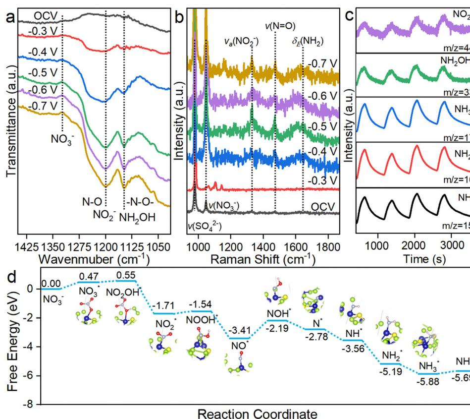
Fig. 4 (a) Electrochemical *in situ* FTIR spectra and (b) *in situ* Raman spectra of S-CoSe<sub>2</sub> NWs. (c) Online DEMS of S-CoSe<sub>2</sub> NWs under a potential of  $-0.35\text{ V}$  vs. RHE. (d) Reaction-free energies for different intermediates of NARR based on the model of sulfur-doped  $\text{CoSe}_2$ .
