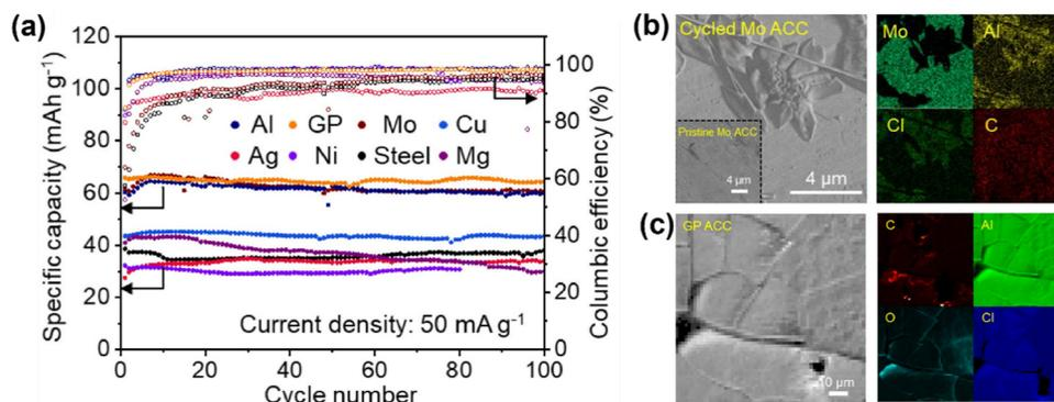
Fig. 10 Electrochemical measurements and *ex situ* characterization of different anodic CCs. (a) Cycling performance of different anodic CCs at a fixed rate of  $50 \text{ mA g}^{-1}$  (b) SEM and EDX measurements of fully discharged Mo anodic CC after 100 cycles. (c) AES image and corresponding AES elemental mapping of fully charged GP anodic CC etched for 20 min by argon ion bombardment. Reprinted with permission,<sup>128</sup> Elsevier, Copyright 2022.
