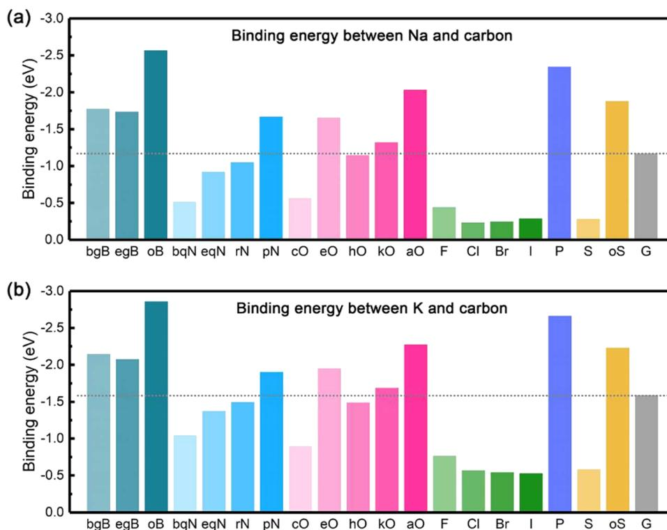
Fig. 2 The summary of binding energy on carbon materials: (a) the binding energy between Na and carbon, (b) the binding energy between K and carbon. Reprinted with permission,<sup>37</sup> Elsevier, Copyright 2020.
