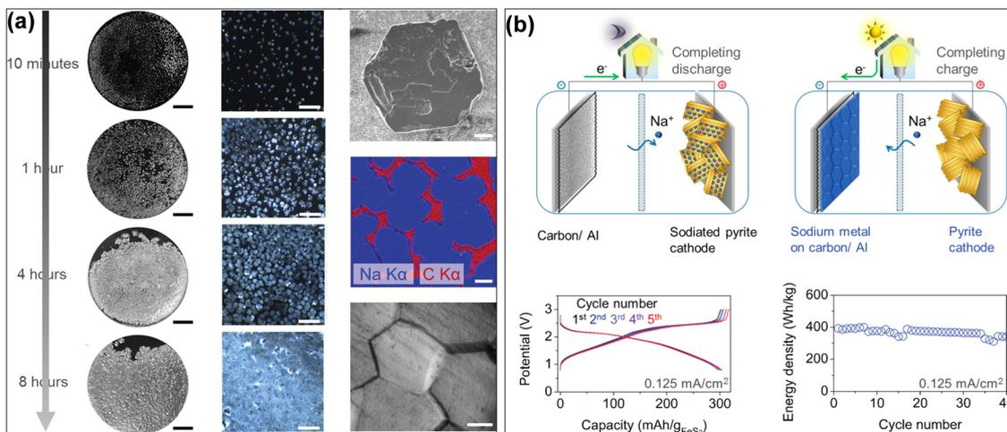
Fig. 4 (a) Photographs and micrographs of metallic Na on C/Al electrodes at  $0.5 \text{ mA cm}^{-2}$ , and also SEM and micrograph images of hexagon-shaped Na metal islands. (b) Schematic illustration of the charge/discharge process of the C/Al CC (anode) with sodiated pyrite cathode in a AFSMB cell, and some electrochemical results. Reprinted with permission,<sup>53</sup> American Chemical Society, Copyright 2017.
