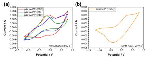
Fig. 3 Cyclic voltammograms of (a) positive electrode materials, PPy(PSS), PPy(SS), and PPy(DBS) and (b) a negative electrode material, PPy(ClO<sub>4</sub>) in the 10 mM NaCl solution with a scan rate of 2 mV s<sup>-1</sup>; the potentials are against Ag/AgCl.
