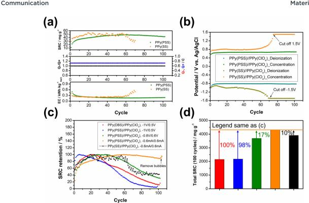
Fig. 5 (a) Comparisons between the salt removal capacity (SRC) profile, Q-/Q+ value, and energy consumption (EC) profile for PPy(PSS)//PPy(ClO<sub>4</sub>) and PPy(SS)//PPy(ClO<sub>4</sub>) with deionization, concentration = -0.6 mA/0.6 mA, 20 min/20 min. (b) The potential profile during the operation in (a). (c) The retention comparison of all systems. (d) Accumulated SRC after 100 cycles for all systems.
