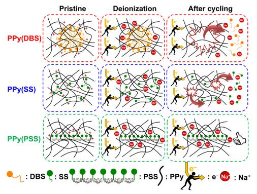
Fig. 7 Schematic of the degradation mechanism of PPy(DBS) with large micelles formation, PPy(SS) with no micelle formation or incomplete micellelike structures formation, and PPy(PSS) with no micelle formation.
