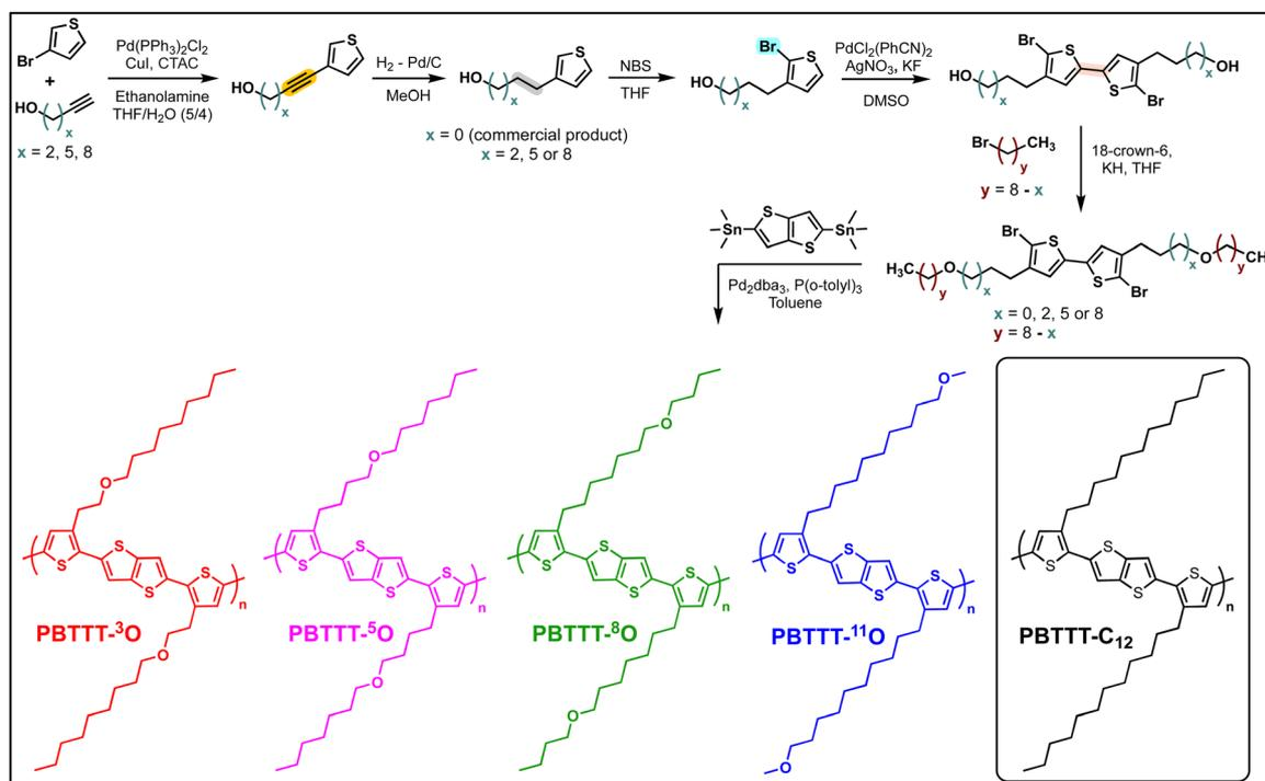
Scheme 1 General synthetic route towards the ether-based PBTTT-<sup>x</sup>O. In inset, PBTTT-C<sub>12</sub> structure.
