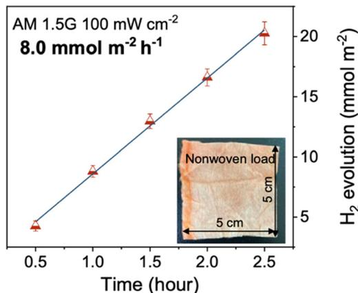
Fig. 24 Photocatalytic rate of PTA film prepared on non-woven fabric (inset). Reprinted under CC-BY 4.0 License.<sup>171</sup>
