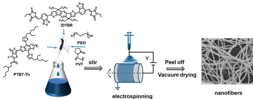
Fig. 15 The electrospinning process used to prepare D–A nanofibers. Reprinted under CC-BY 4.0 License.<sup>48</sup>
