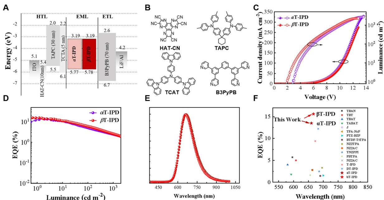
Fig. 4 (A) OLED structure, HOMO and LUMO energy diagram. (B) The material structure used in the functional layer, (C) current density ( $J$ )–voltage curves ( $V$ )–luminance ( $L$ ), (D) EQE– $L$  curves, and (E) EL spectra of non-doped OLEDs based on  $\alpha$ T-IPD and  $\beta$ T-IPD. (F) Reported representative hot exciton DR-OLEDs.
