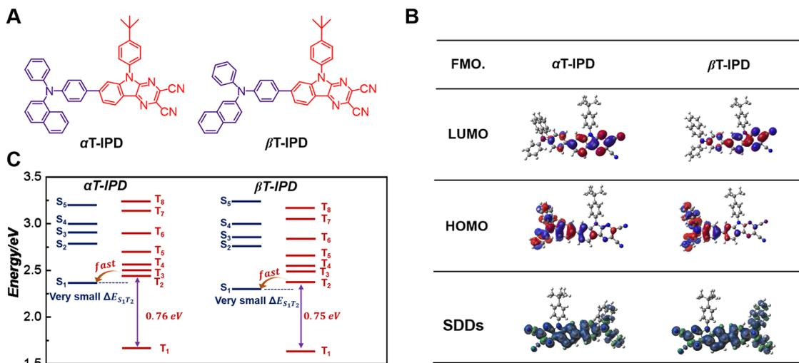
Fig. 1 (A) The chemical structures of  $\alpha$ T-IPD and  $\beta$ T-IPD. (B) HOMO and LUMO, and  $T_1$  states spin-density distributions (TSDs) of  $\alpha$ T-IPD and  $\beta$ T-IPD, respectively. (C) Calculated energy arrangement of singlet states and triplet states of  $\alpha$ T-IPD and  $\beta$ T-IPD.
