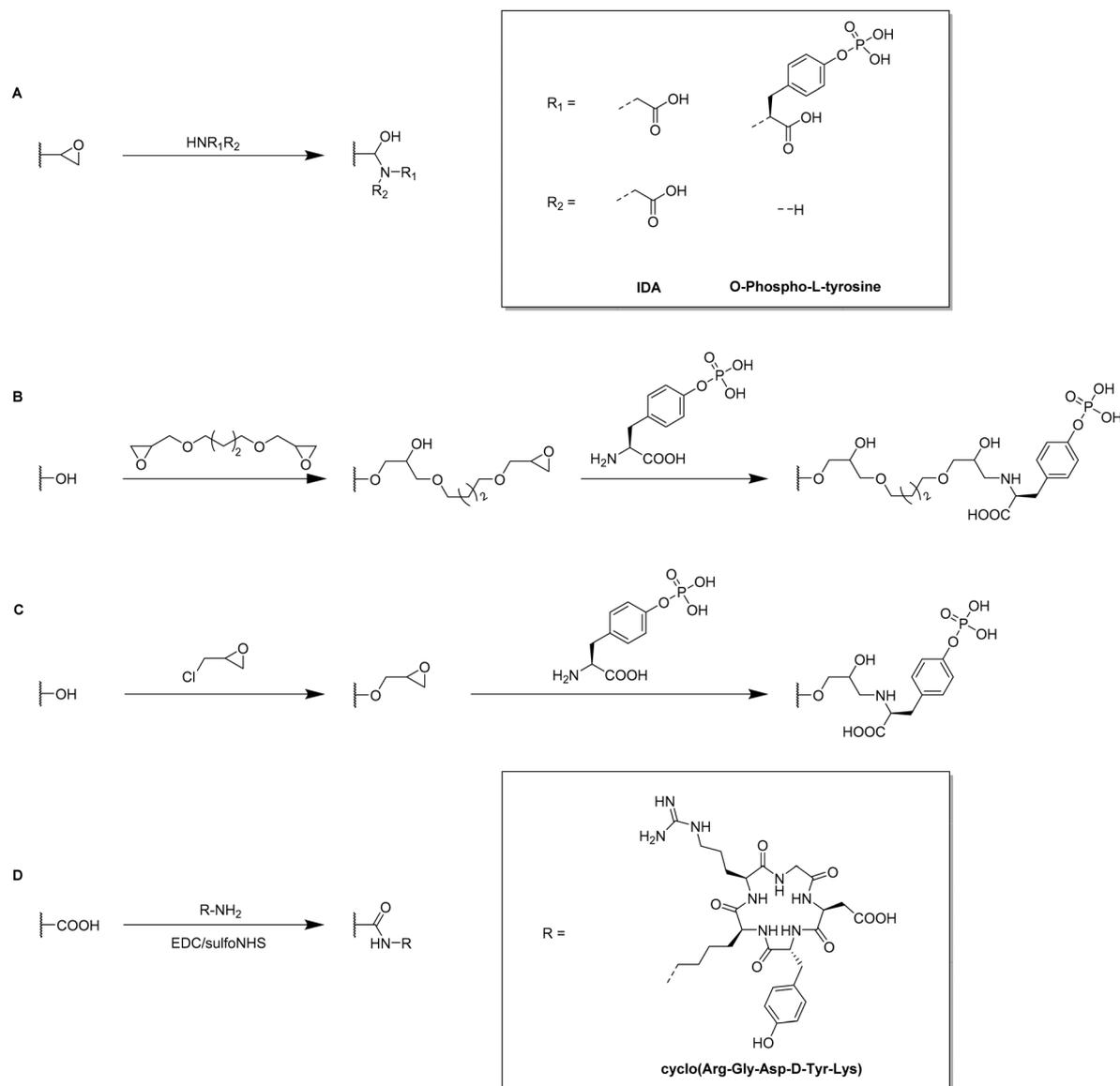
Fig. 35 Schematic representation of the subsequent modification of hybrid cryogels by the direct functionalization of epoxide groups with amines such as IDA or *o*-phospho-L-tyrosine (A), or *via* the modification of hydroxy groups by the introduction of epoxy groups using 1,4-butanedioldiglycidyl ether (B) or epichlorohydrin (C). Alternative strategies include the attachment of peptides such as cyclo(Arg-Gly-Asp-D-Tyr-Lys) *via* EDC/sulfoNHS coupling towards cryogel carboxylic acid groups (D).
