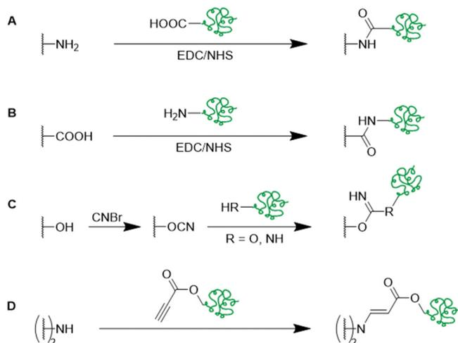
**Fig. 23** Schematic representation of alternative functionalization strategies of synthetic polymer based cryogels with biopolymers e.g. enzymes, proteins and polysaccharides *via* EDC coupling (A) and (B), cyanogen bromide activation (C) of cryogel hydroxy groups or using amino-yne click reaction (D).
