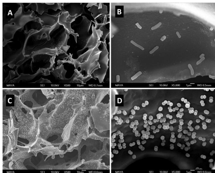
Fig. 16 SEM images of multiple boronic acid ligands containing cryogels with bound *E. coli* (A) and (B) and *S. epidermidis* (C) and (D) on. The scale bars are 10 µm in (A) and (C) and 1 µm in (B) and (D). Reproduced under terms of the CC-BY license with permission.<sup>58</sup> Copyright 2022, The Authors, published by the American Chemical Society.
