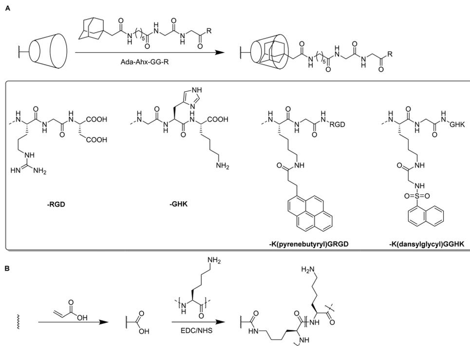
**Fig. 19** Schematic representation of various strategies for the functionalization of synthetic polymer based cryogels with peptides. Functionalization of  $\beta$ -CD containing cryogels via host-guest interaction with adamantyl-coupled peptide sequences (A). Introduction of acid groups by photo-induced graft polymerization followed by *p*(L-lysine) attachment (B).
