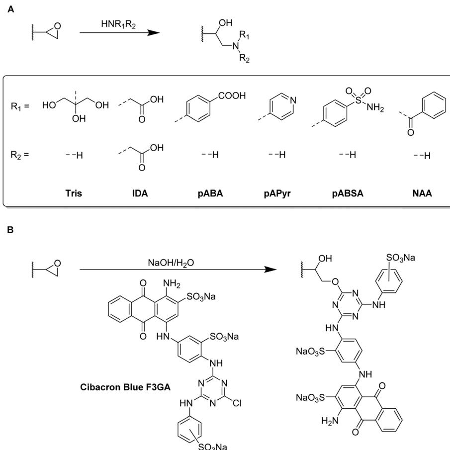
**Fig. 13** Schematic representation of the direct functionalization of synthetic polymer based cryogels with amine containing small functional molecules (A) such as tris(hydroxymethyl)aminomethane (Tris), iminodiacetic acid (IDA), *para*-amino benzoic acid (pABA), *para*-amino pyridine (pAPyr), *para*-amino benzenesulfonamide (pABSA) and nicotinamide (NAA), or cibacron blue F3GA (B) via the direct coupling towards epoxides on cryogel surfaces.
