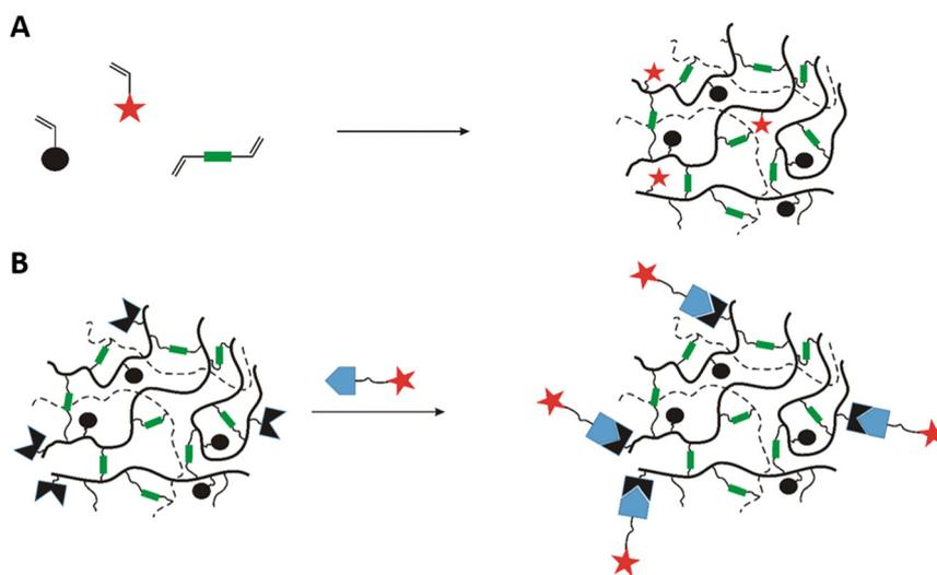
**Fig. 11** Schematic representation of the preparation of functionalized cryogels based on synthetic polymers using either free radical cross-linking polymerization of functional monomers (A) or *via* modification with small molecules, biomolecules and biopolymers (B).
