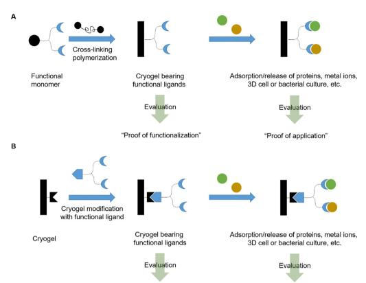
Fig. 1 Schematic representation of the functionalization of cryogels by the use of functional monomers (A) or by the subsequent modification of cryogels with functional ligands (B) for the adsorption of target molecules such as proteins or heavy metal ions.
